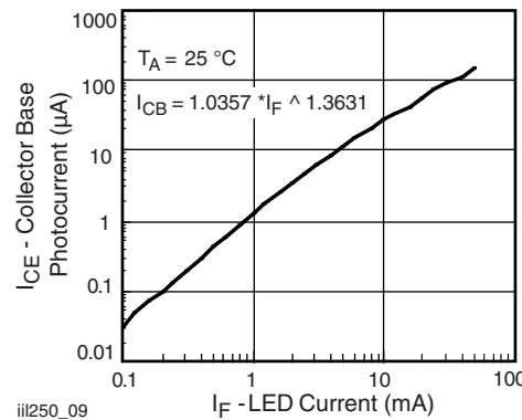
Fig. 9 - Collector Base Photocurrent vs. LED Current
