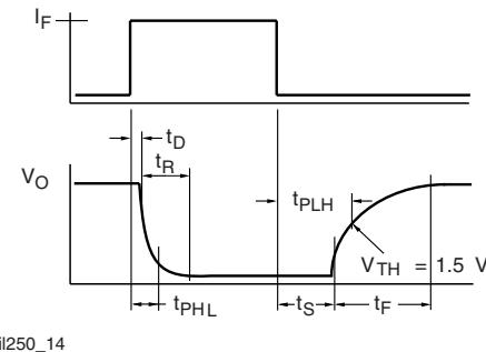
Fig. 14 - Switching Timing
