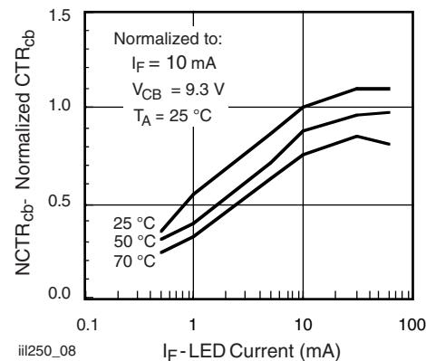
Fig. 8 - Normalized CTR<sub>CB</sub> vs. LED Current and Temperature
