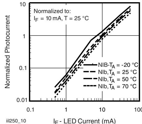
Fig. 10 - Normalized Photocurrent vs. I\_F and Temperature
