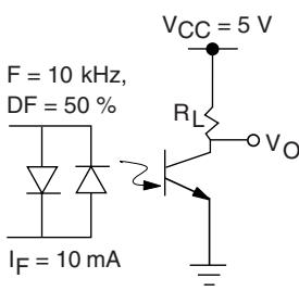
Fig. 15 - Switching Schematic
