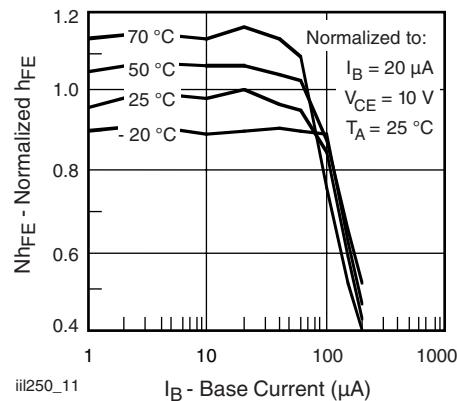
Fig. 11 - Normalized Non Saturated  $h_{FE}$  vs.
