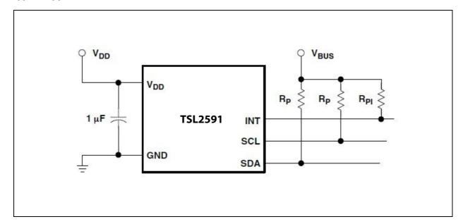
The I²C signals and the Interrupt are open-drain outputs and require pull-up resistors. The pull-up resistor (RP) value is a function of the I²C bus speed, the I²C bus voltage, and the capacitive load. The ams EVM running at 400 kbps, uses 1.5-k $\Omega$  resistors. A 10-k $\Omega$  pull-up resistor (RPI) can be used for the interrupt line.
