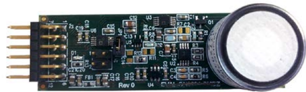
Figure 5. EVAL-CN0357-PMDZ Evaluation Board
