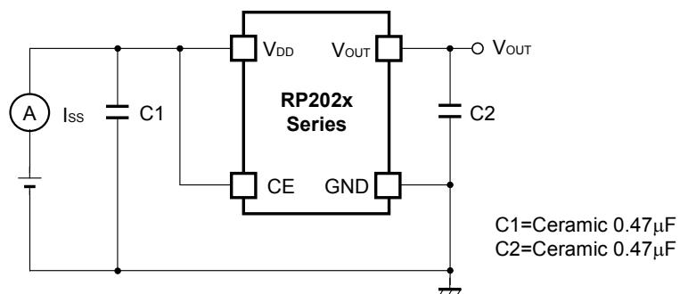
**Test Circuit for Supply Current**
