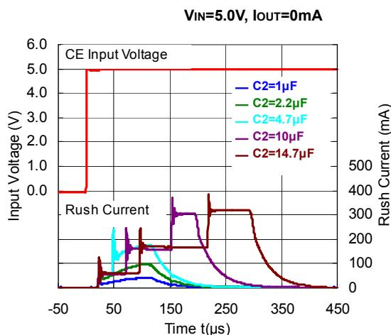
16) Turn On Speed with CE pin (D Version) ( $C_1=0.47\mu F$ ,  $C_2=0.47\mu F$ ,  $T_a=25^{\circ}C$ )
