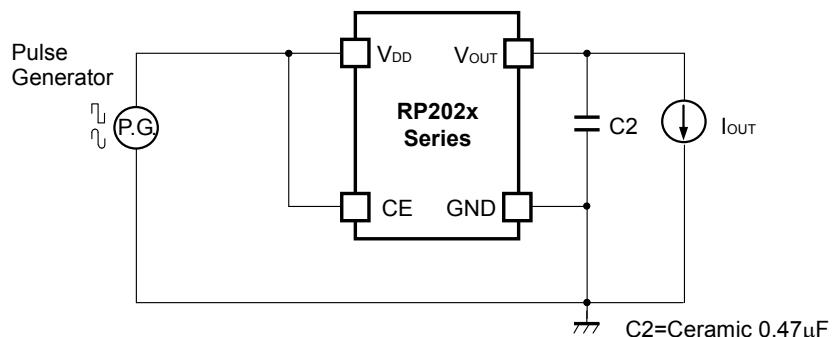
**Test Circuit for Ripple Rejection**
