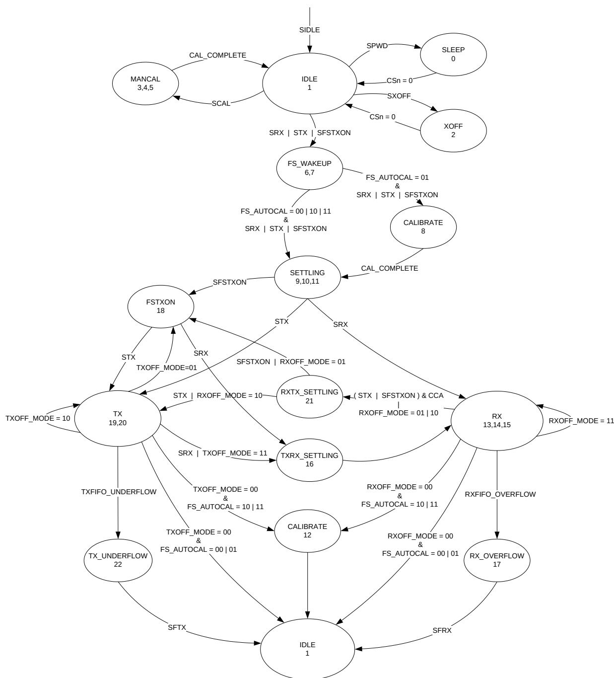
Figure 19: Complete Radio Control State Diagram
