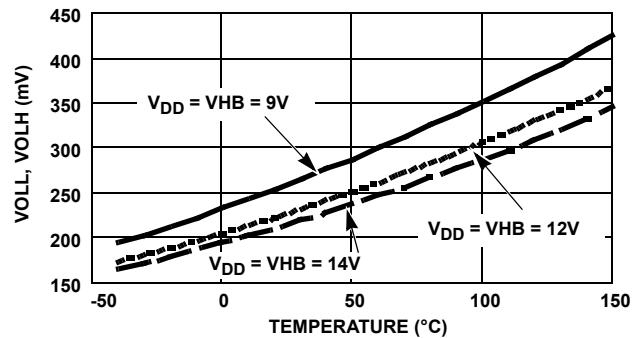
FIGURE 10. LOW LEVEL OUTPUT VOLTAGE vs TEMPERATURE
