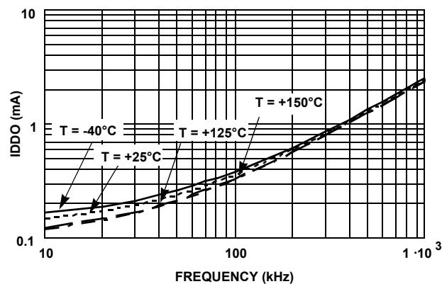
FIGURE 5. ISL2100A IDD OPERATING CURRENT vs FREQUENCY
