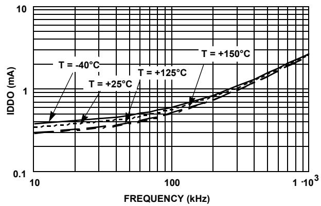
FIGURE 6. ISL2101A IDD OPERATING CURRENT vs FREQUENCY
