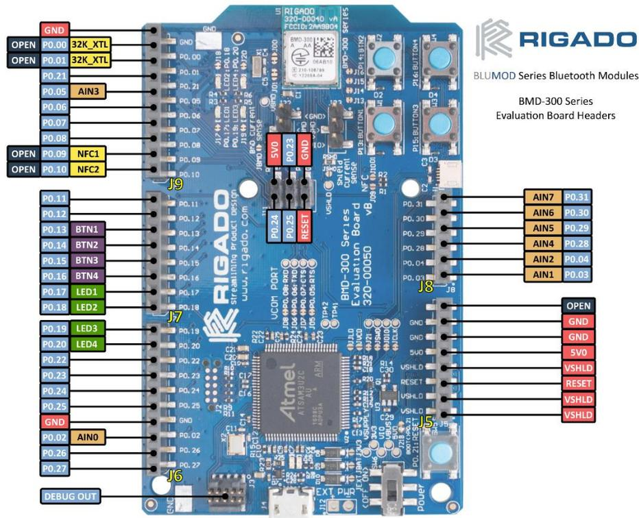
Figure 18 – BMD-300 Series Evaluation Board Pin-out
