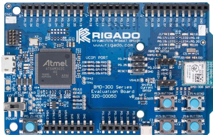
Figure 1 – BMD-300 Evaluation Board (Top View)
