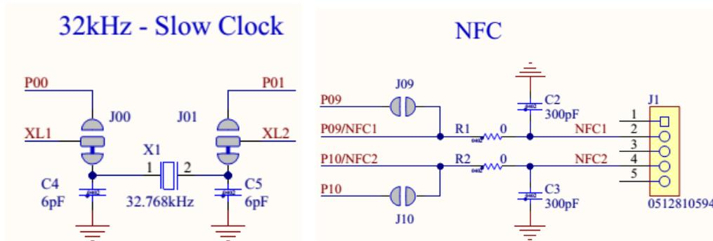
Figure 16 – GPIOs disconnected from I/O headers
