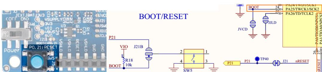
Figure 9 – Schematic – Reset
