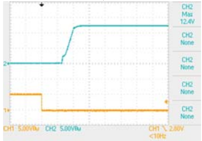
Stepload Transient Response (Vin = 24V, Iout = 50-75-50% of Imax, Cload = 470µF, Io = 200mA/div, Ta = +25°C) CH2 = Vout, CH4 = Iout
