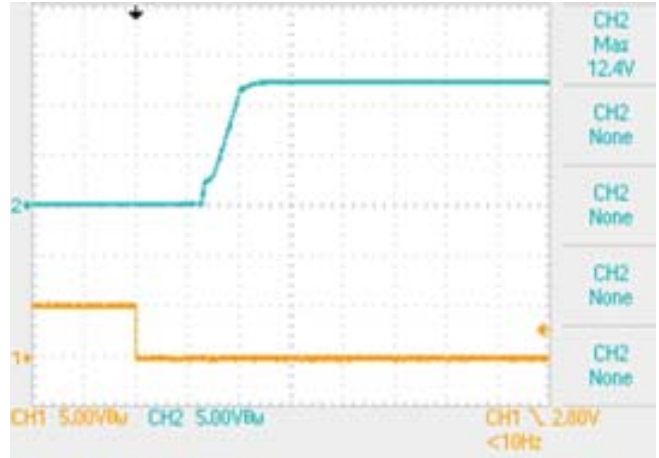
Stepload Transient Response ( V_{in} = 24V , I_{out} = 50-75-50\% of I_{max} , Load = 470\mu F , I_o = 200mA/div , T_a = +25^\circ C ) CH2 = Vout, CH4 = Iout
