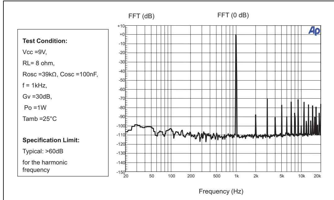
**Figure 23. FFT (-60 dB)**
