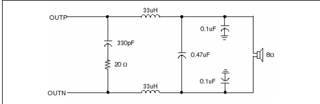
**Figure 33. Typical LC filter for a 4- $\Omega$  speaker**
