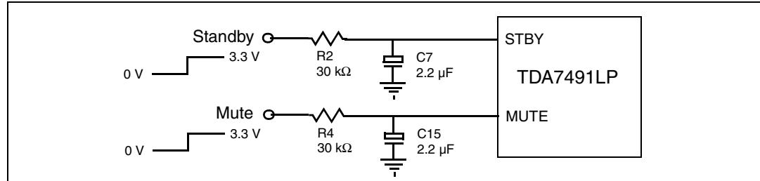
**Figure 28. Turn-on/off sequence for minimizing speaker “pop”**
