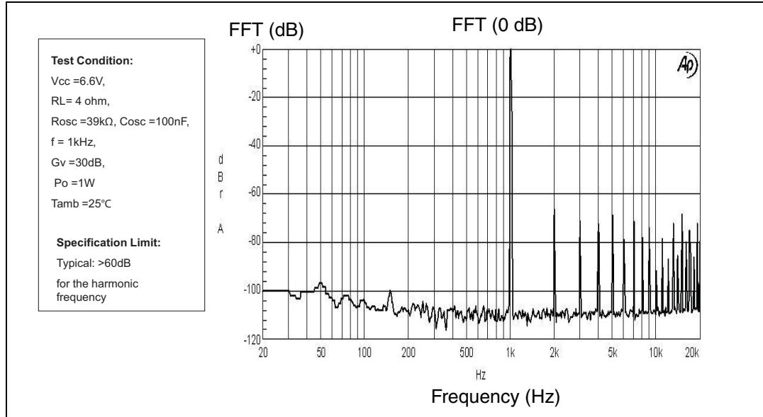
**Figure 10. FFT (-60 dB)**
