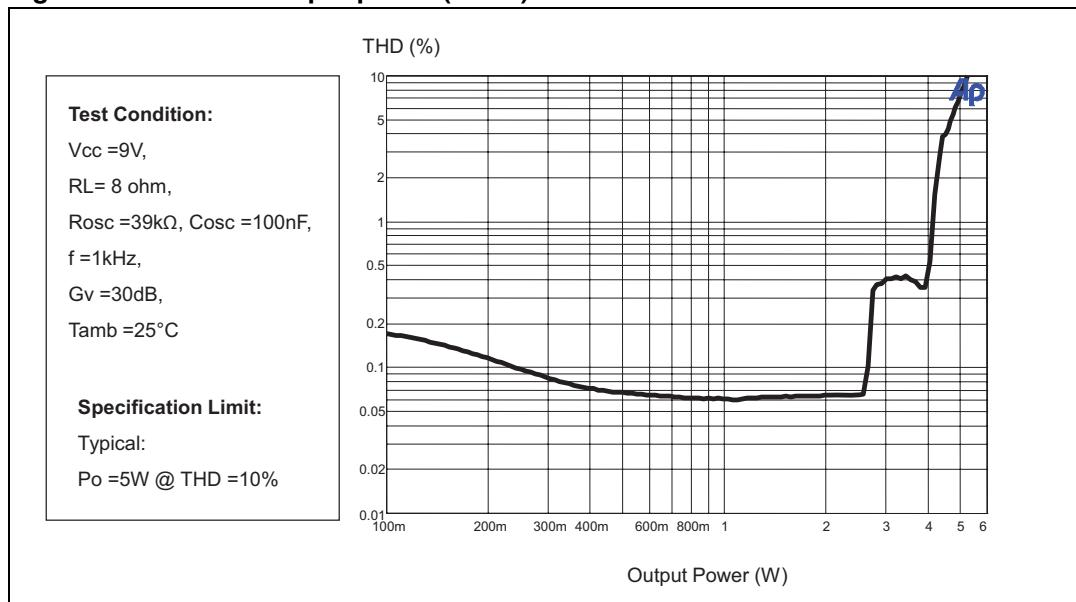
**Figure 18. THD vs. output power (100 Hz)**
