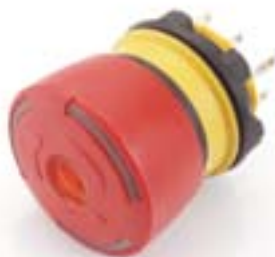
Emergency-stop red LED illuminated, plug-in terminals, twist release, 32mm diameter for 22.5mm mounting, foolproof to EN 60947-5-5, EN418
