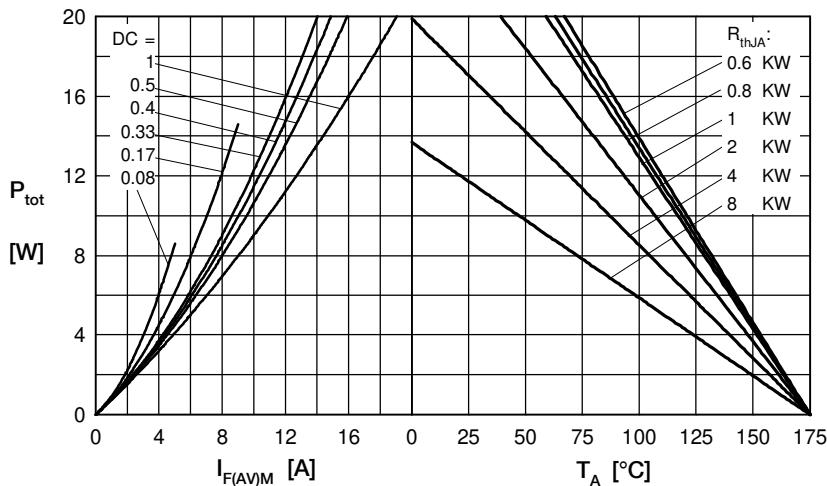
Fig. 4 Power dissipation vs. forward current
