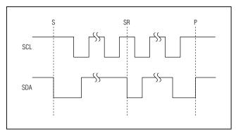
Figure 4. START, STOP, and Repeated START Conditions
