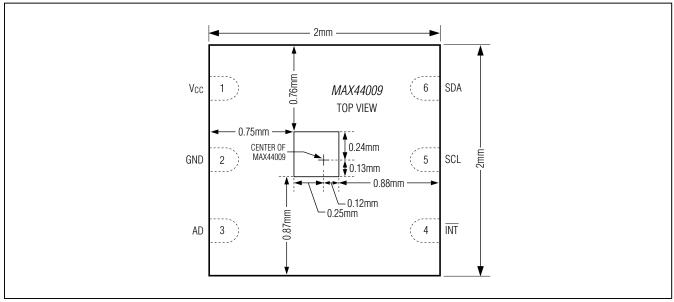
Figure 9. Sensor Position
