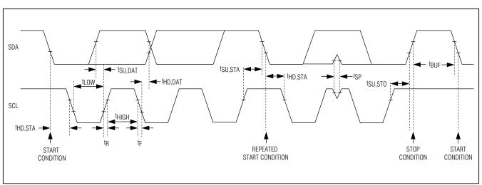
Figure 3. 2-Wire Interface Timing Diagram
