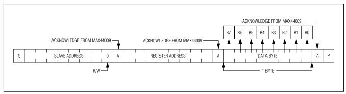
Figure 6. Writing 1 Byte of Data to the IC
