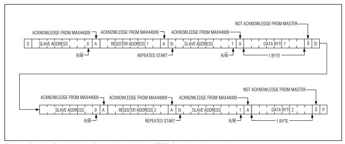
Figure 8. Reading Two Registers Consecutively Without a STOP Condition in Between Reads
