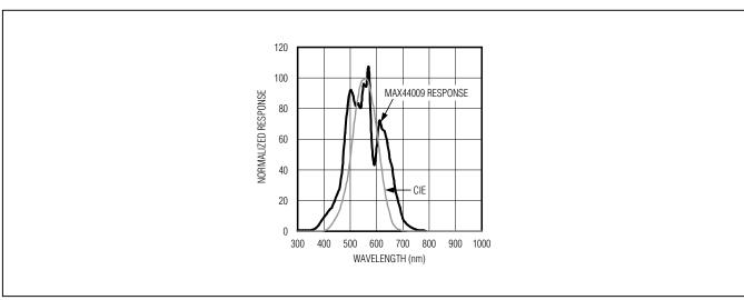
Figure 1. Spectral Sensitivity of the MAX44009 and Human Eye
