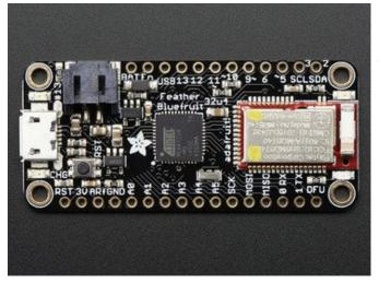
Bluefruit Micro or Feather 32u4 Bluefruit If you have a Bluefruit Micro or Feather 32u4 Bluefruit LE then you have an ATmega32u4 chip with Hardware SPI, CS = 8, IRQ = 7, RST = 4
