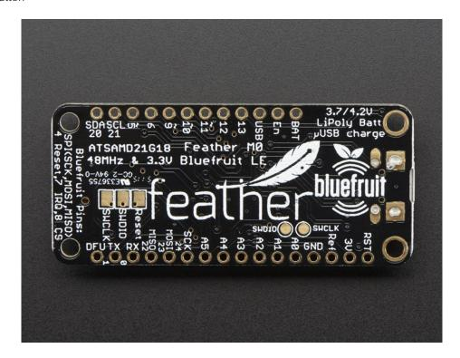
The Feather M0 Bluefruit uses the extra space left over to add our excellent Bluefruit BTLE module + two status indicator LEDs
