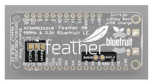
The round pads on the right are for the ATSAMD21G18 (main processor). The rectangular pads to the left are for the nrf51822 inside the BLE module.
