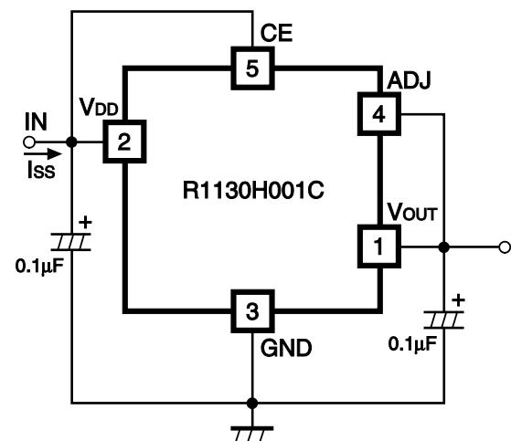
Fig.2 Test Circuit Supply Current
