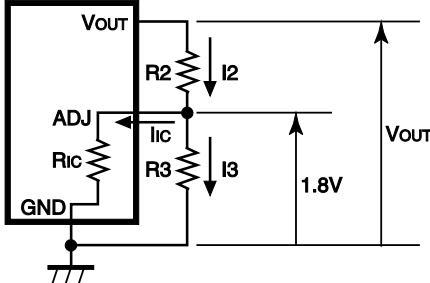
The Output Voltage of Regulator in R1130xxxxC may be adjustable for any output voltage between its 1.8V reference and its  $V_{DD}$  setting level. An external pair of resistors is required, as shown in Figure 1.
