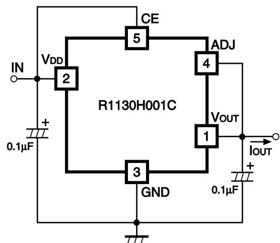
Fig.1 Standard test Circuit
