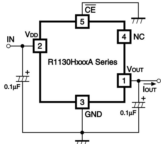
Fig.1 Standard test Circuit
