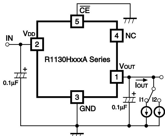
Fig.4 Load Transient Response Test Circuit
