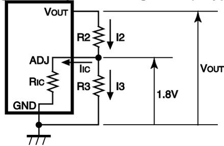
The Output Voltage of Regulator in R1130xxxxC may be adjustable for any output voltage between its 1.8V reference and its V<sub>DD</sub> setting level. An external pair of resistors is required, as shown in Figure 1.
