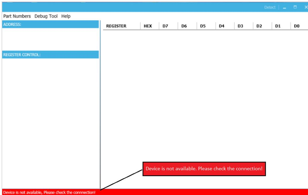
**Figure 9: Warning Indicates Unsuccessful Connection – USBI2C Dongle is Not Connected**
