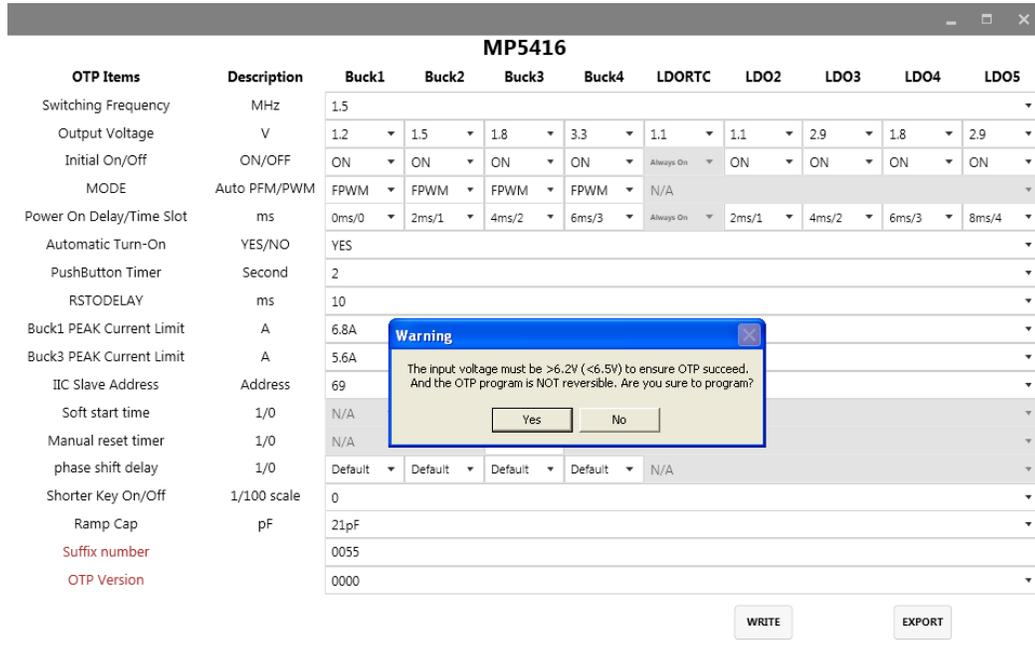
**Figure 17: Important Warning – User Must Increase Voltage**
