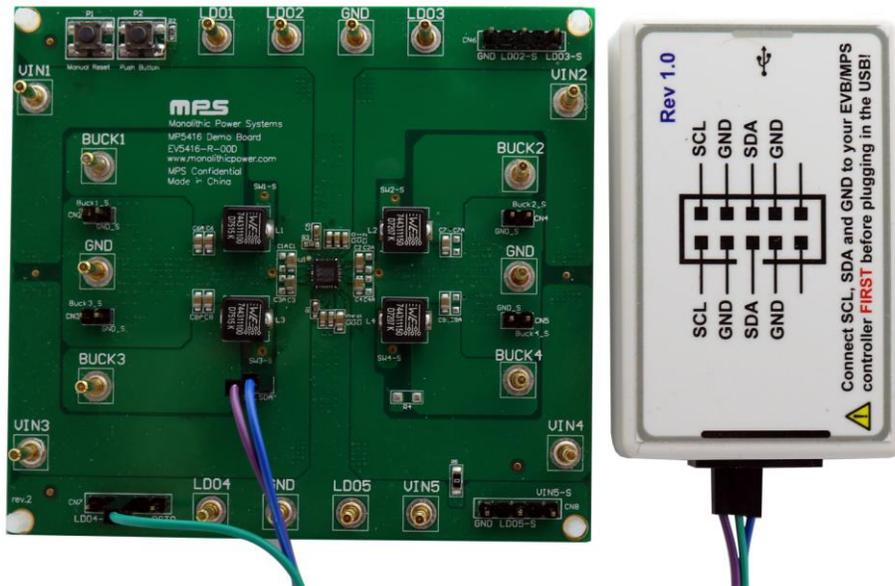
**Figure 6: EVB to MPS I<sup>2</sup>C Dongle Wire Connection**
