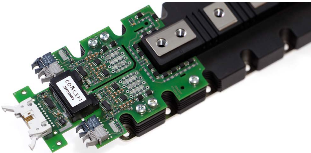
Fig. 1 2SP0320V screwed onto a PrimePACK™ IGBT module
