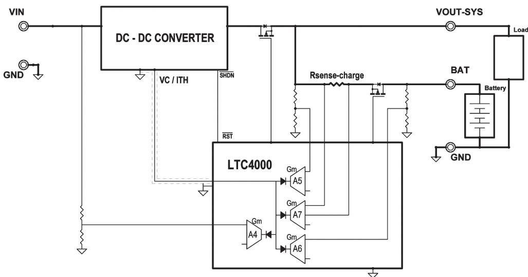
Figure 2. Block Diagram with Typical DC/DC Converter
