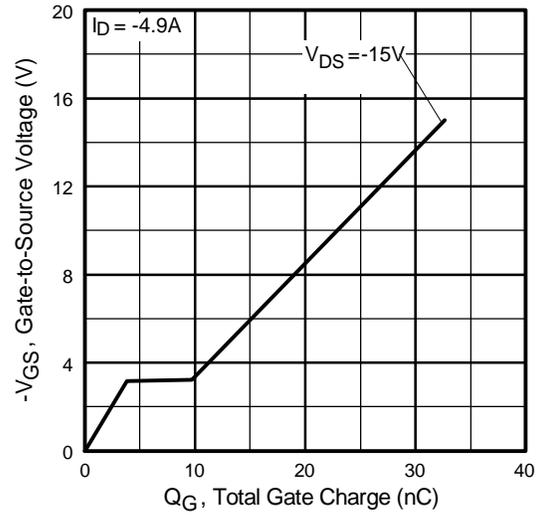
**Fig 21.** Typical Gate Charge Vs. Gate-to-Source Voltage
