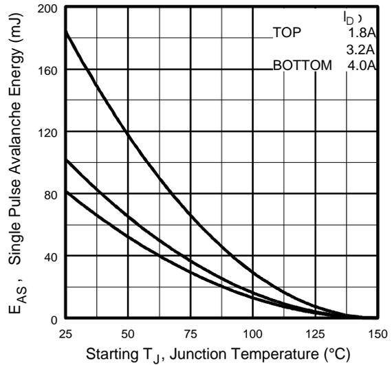
**Fig 8.** Maximum Avalanche Energy Vs. Drain Current
