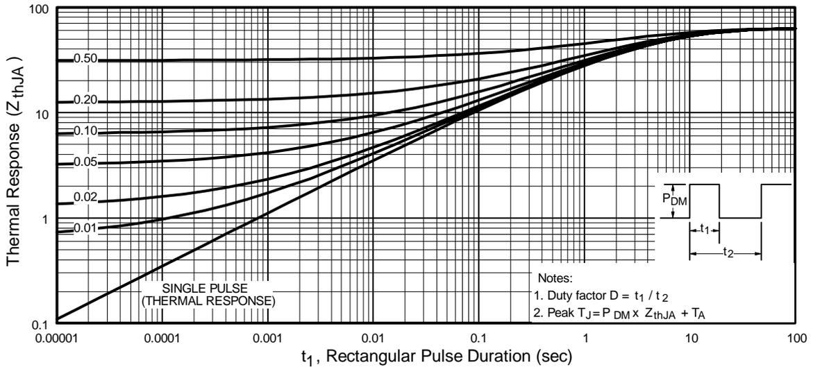
**Fig 22.** Maximum Effective Transient Thermal Impedance, Junction-to-Ambient
