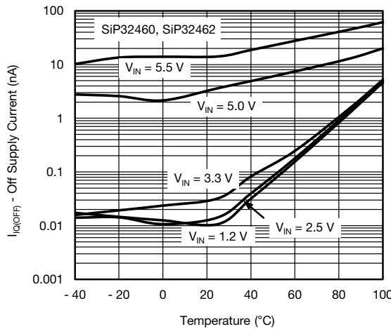
Fig. 9 - Off Supply Current vs. Temperature
