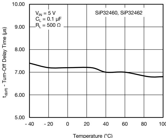
Fig. 21 - Turn-off Delay Time vs. Temperature
