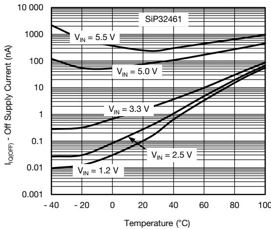
Fig. 6 - Off Supply Current vs. Temperature
