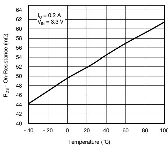
Fig. 14 -  $R_{DS(\text{on})}$  vs. Temperature
