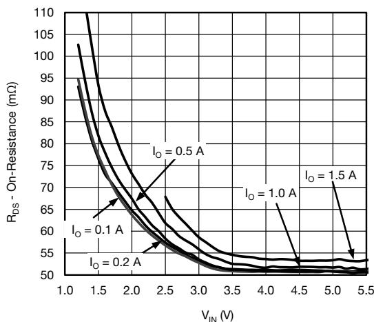
Fig. 11 -  $R_{DS(\text{on})}$  vs. Input Voltage
