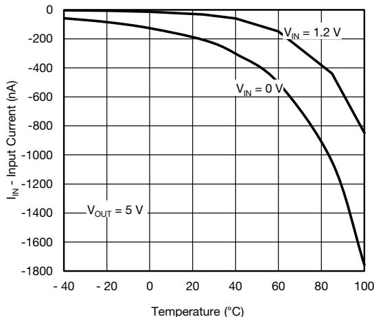
Fig. 16 - Reverse Blocking Current vs. Temperature
