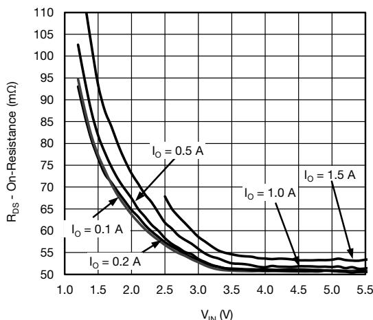
Fig. 11 -  $R_{DS(\text{on})}$  vs. Input Voltage
