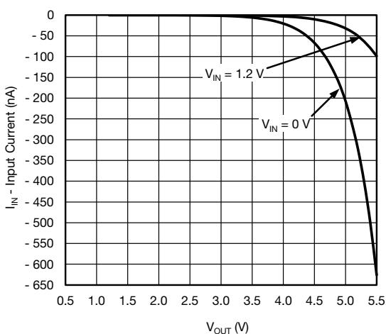
Fig. 12 - Reverse Blocking Current vs. Output Voltage
