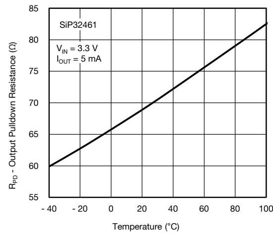
Fig. 23 - Output Pulldown Resistance vs. Temperature
