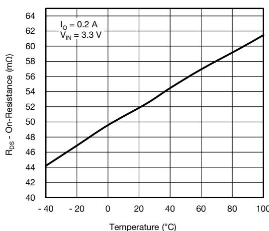
Fig. 14 -  $R_{DS(\text{on})}$  vs. Temperature
