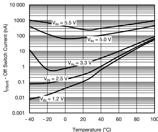
Fig. 13 - Off Switch Current vs. Temperature
