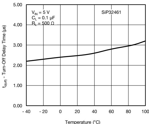
Fig. 22 - Turn-off Delay Time vs. Temperature
