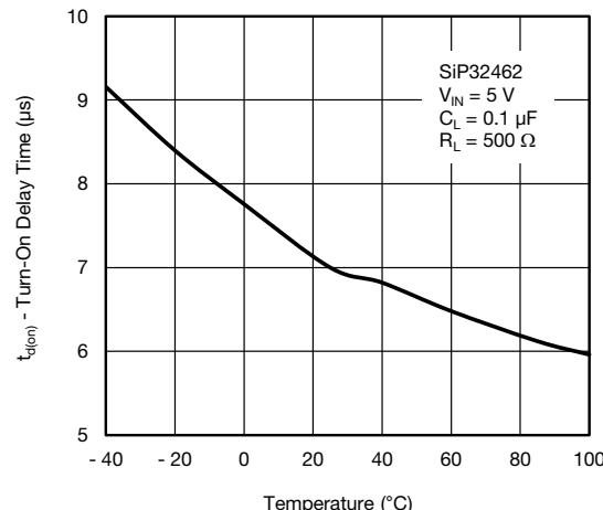
Fig. 19 - Turn-on Delay Time vs. Temperature
