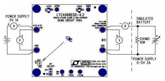
Figure 1. Proper Measurement Equipment Setup
