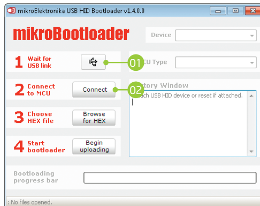
Figure 3-3: USB HID mikroBootloader window
