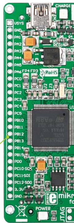
Most microcontroller pins are available for further connectivity via two 1x26 rows of connection pads on both sides of the mikromedia board. They are designed to match additional shields, such as Battery Boost shield, Gaming, PROTO shield and others.
