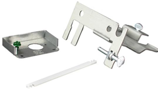
Accessory pack for 25 Series and AM Series poles. Includes two ceiling trim plates, hanger clamp assembly, feed end fitting, and floor mounting assembly. One Accessory Pack supplied with each Tele-Power pole at no extra charge. Boots are not offered in accessory packs.
