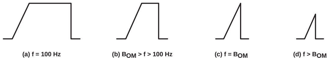
Figure 5. Full-Power-Response Output Signal
