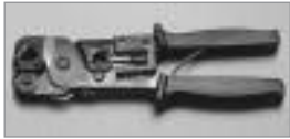
Modular Crimping Tool that cuts, strips and terminates 4, 6, 8, & 8 Keyed Modular Plugs. (Works on AMP™ & Stewart™ Plugs.)
