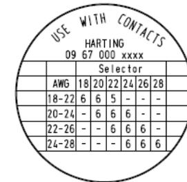
Note that the new locator 09 99 000 0531 is equivalent to the old locator 61 03 600 0024. Only the label on the top has been changed (see above right label). The locator 61 03 600 0023 should not be used with these new contact part numbers.
