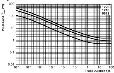
Maximum pulse load, single pulse; applicable if  $\bar{P} \rightarrow 0$  and n < 1000 and  $\hat{U} \leq \hat{U}_{max}$ ; for permissible resistance change equivalent to 8000 h operation
