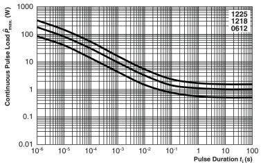
Maximum pulse load, continuous pulses; applicable if  $\bar{P} \leq P \left( \vartheta_{amb} \right)$  and  $\hat{U} \leq \hat{U}_{max}$ ; for permissible resistance change equivalent to 8000 h operation
