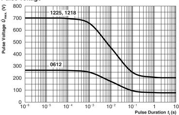
Maximum pulse voltage, single and continuous pulses; applicable if  $\hat{P} \leq \hat{P}_{\text{max}}$  ; for permissible resistance change equivalent to 8000 h operation
