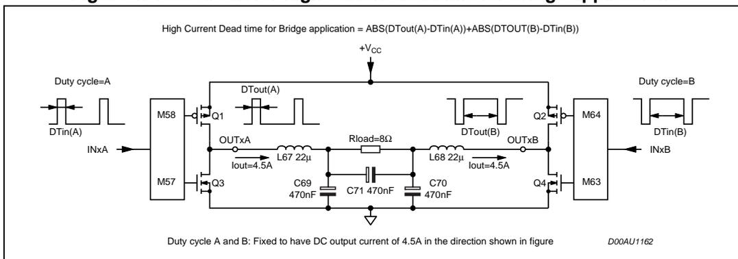
Figure 5. Block diagram for high current dead time for bridge applications
