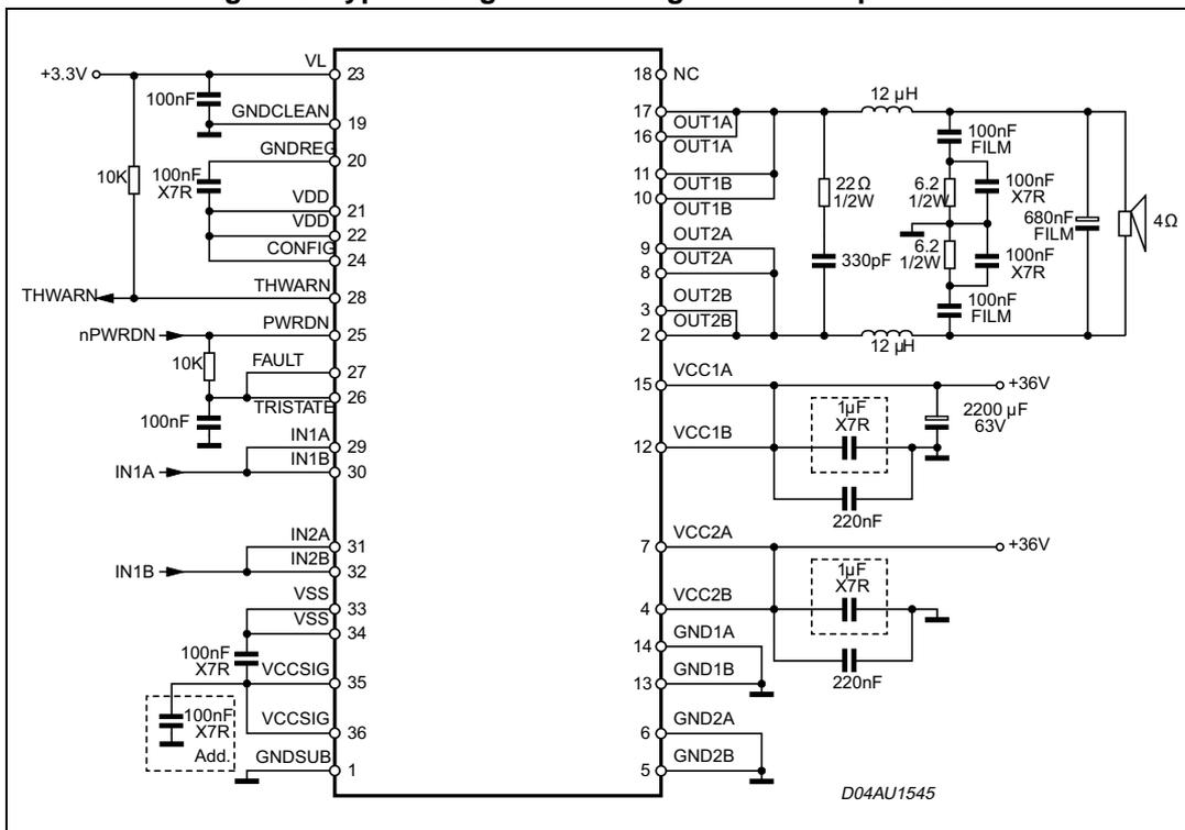
Figure 10. Typical quad half-bridge configuration for up to 4x 50 W
