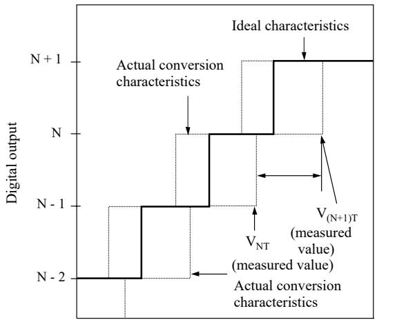
Integral linearity error of digital output N =  $\frac{V_{NT} - \{1 \text{ LSB} \times (N-1) + V_{ZT}\}}{1 \text{ LSB}} \text{ [LSB]}$
