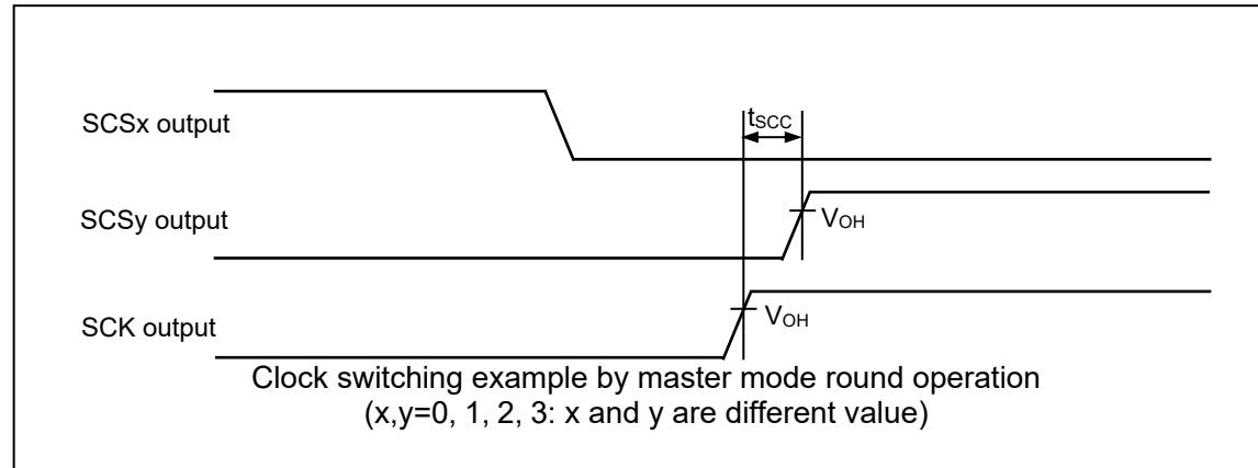
LIN interface (v2.1) (LIN communication control interface (v2.1)) timing (SMR:MD2-0 = 0b011)
