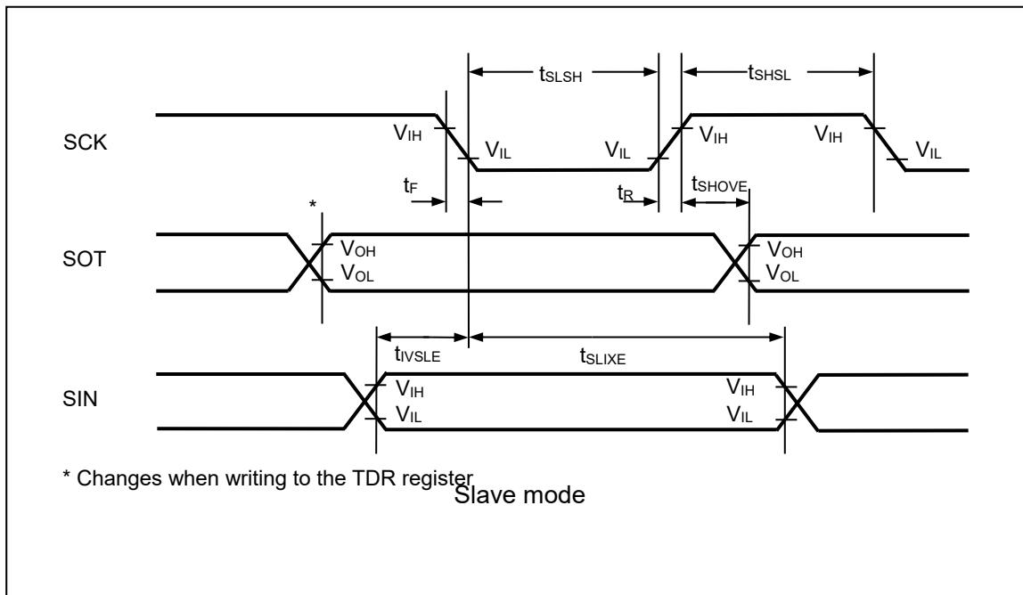
**(4) SPI Supported (SCR:SPI = 1), and Mark Level "L" of Serial Clock Output (SMR:SCINV = 1)**
