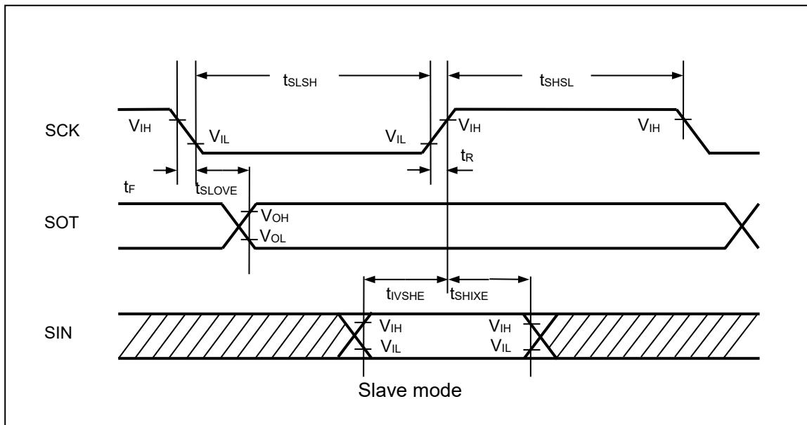
**(2) Normal Synchronous Transfer (SCR:SPI = 0) and Mark Level "L" of Serial Clock Output (SMR:SCINV = 1)**
