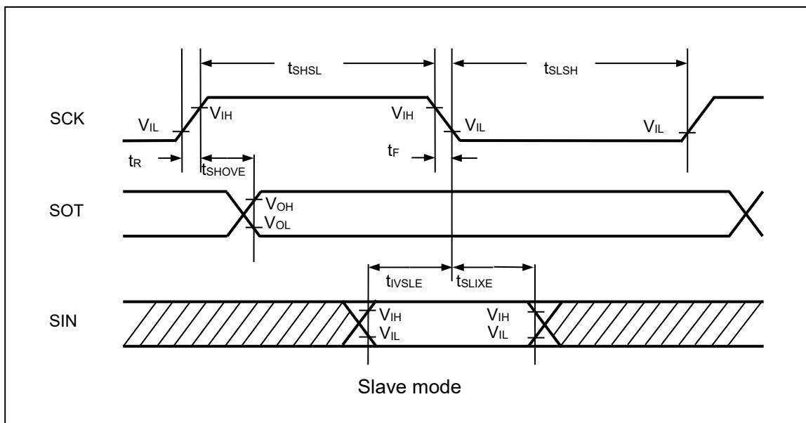
**(3) SPI Supported (SCR:SPI = 1), and Mark Level "H" of Serial Clock Output (SMR:SCINV = 0)**
