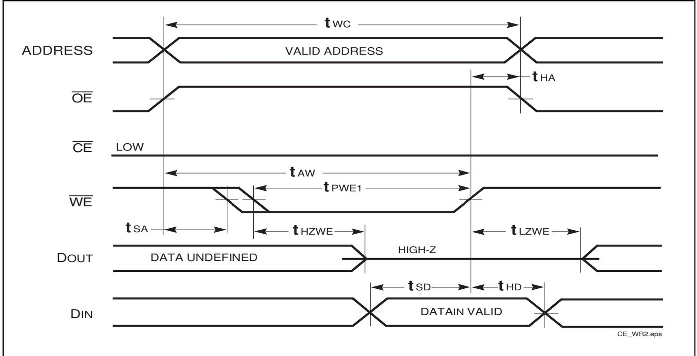
**WRITE CYCLE NO. 3** ( $\overline{OE}$  is LOW During Write Cycle) <sup>(1)</sup>
