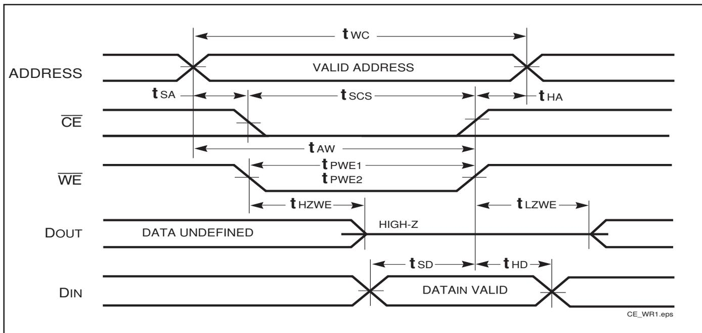
**WRITE CYCLE NO. 2** ( $\overline{OE}$  is HIGH During Write Cycle) <sup>(1,2)</sup>
