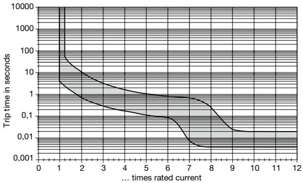
**Curve M2 (medium delay) for AC 50/60 Hz**
