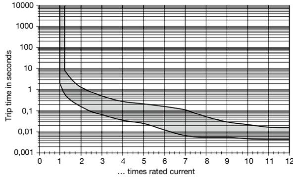
**Curve K2 (short delay) for AC 50/60 Hz**
