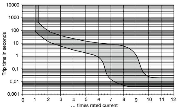
**Curve T2 (long delay) for AC 50/60 Hz**
