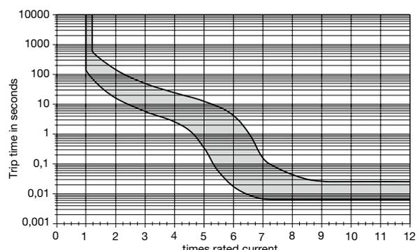
**N.B.** All curves will only be maintained if the escutcheon is mounted on a vertical surface. Ambient temperature or mounting side-by-side does not influence the trip curve, derating is not required. The breakers may trip in the event of current peaks < 0.003 sec. For these applications we offer a mechanical pulse delay – please enquire.
