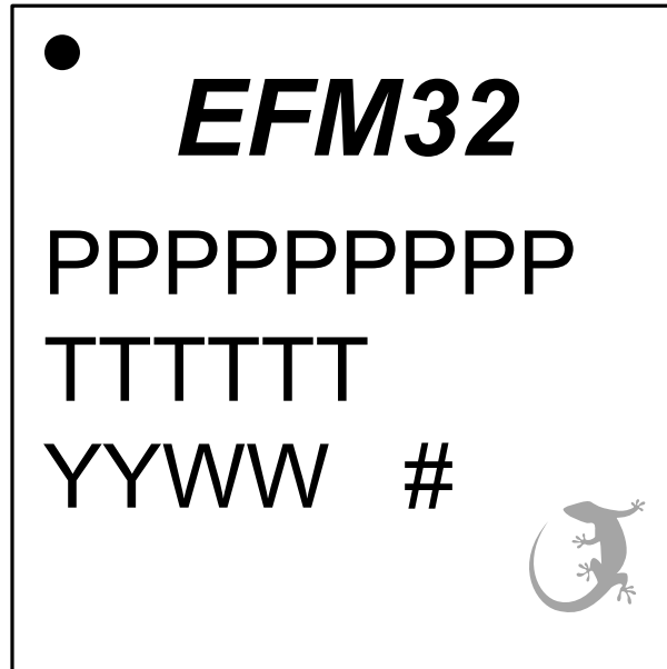
Figure 8.3. QFN32 Package Marking
