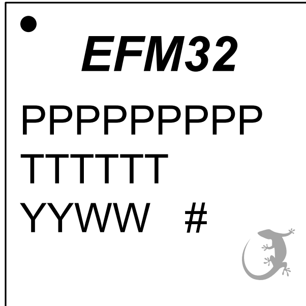
Figure 8.3. QFN32 Package Marking
