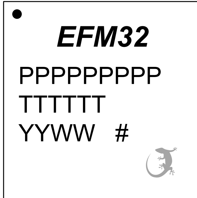
Figure 7.3. QFN48 Package Marking
