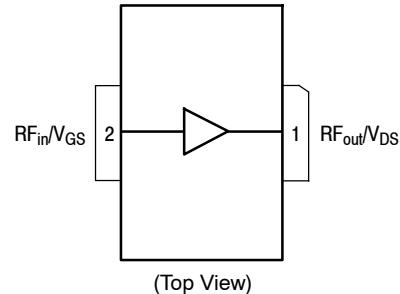
**Figure 1. Pin Connections**
