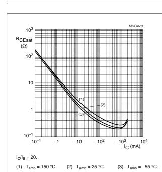
Fig.8 Collector-emitter equivalent on-resistance as a function of collector current; typical values.
