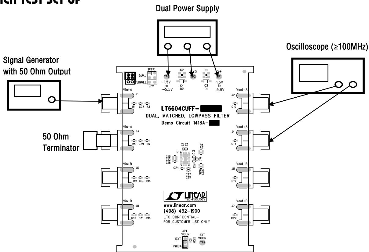
**Figure 2. Dual Supply Test Set Up Connections**
