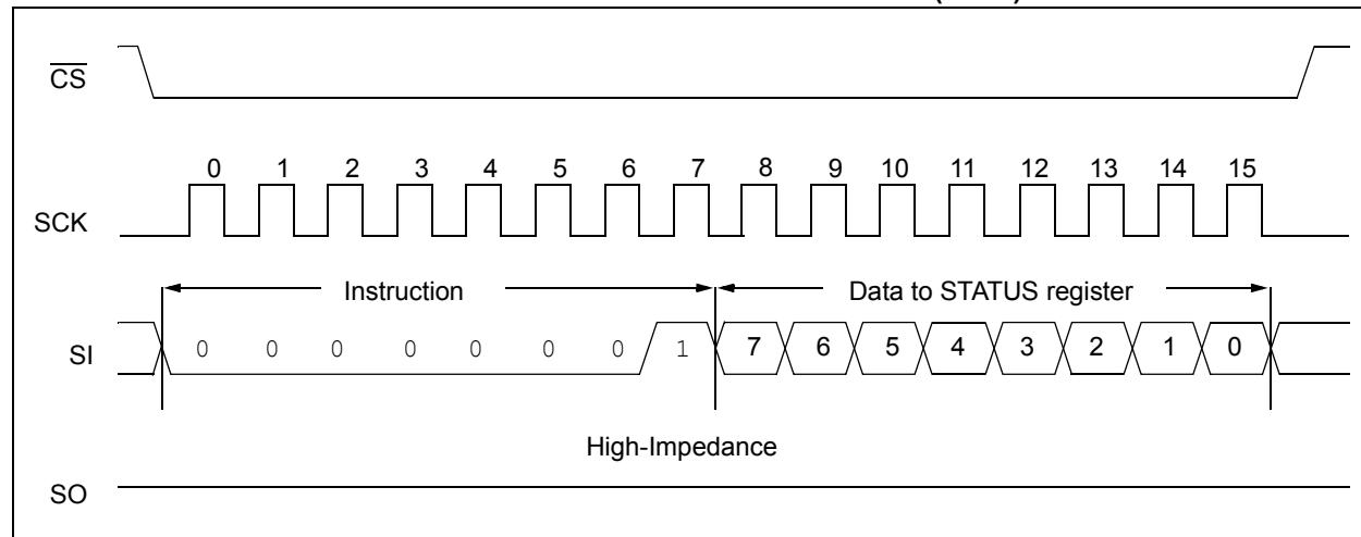
**Note:** An internal write cycle (T<sub>WC</sub>) is initiated on the rising edge of  $\overline{CS}$  after a valid write STATUS register sequence.
