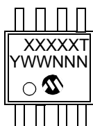
8-Lead MSOP (150 mil)
