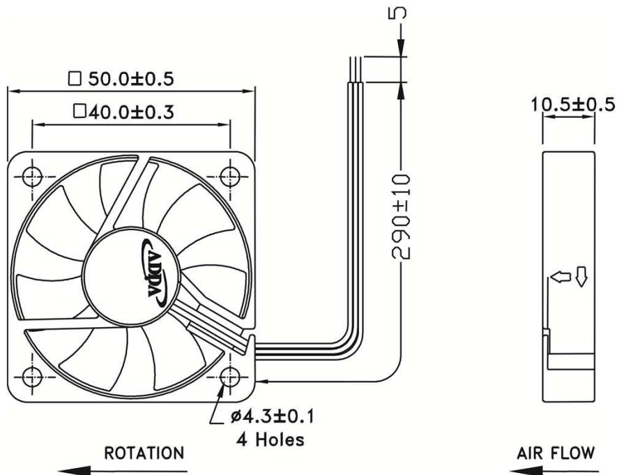
LEAD WIRES : UL 1007, AWG26 , L = 290±10 mm
