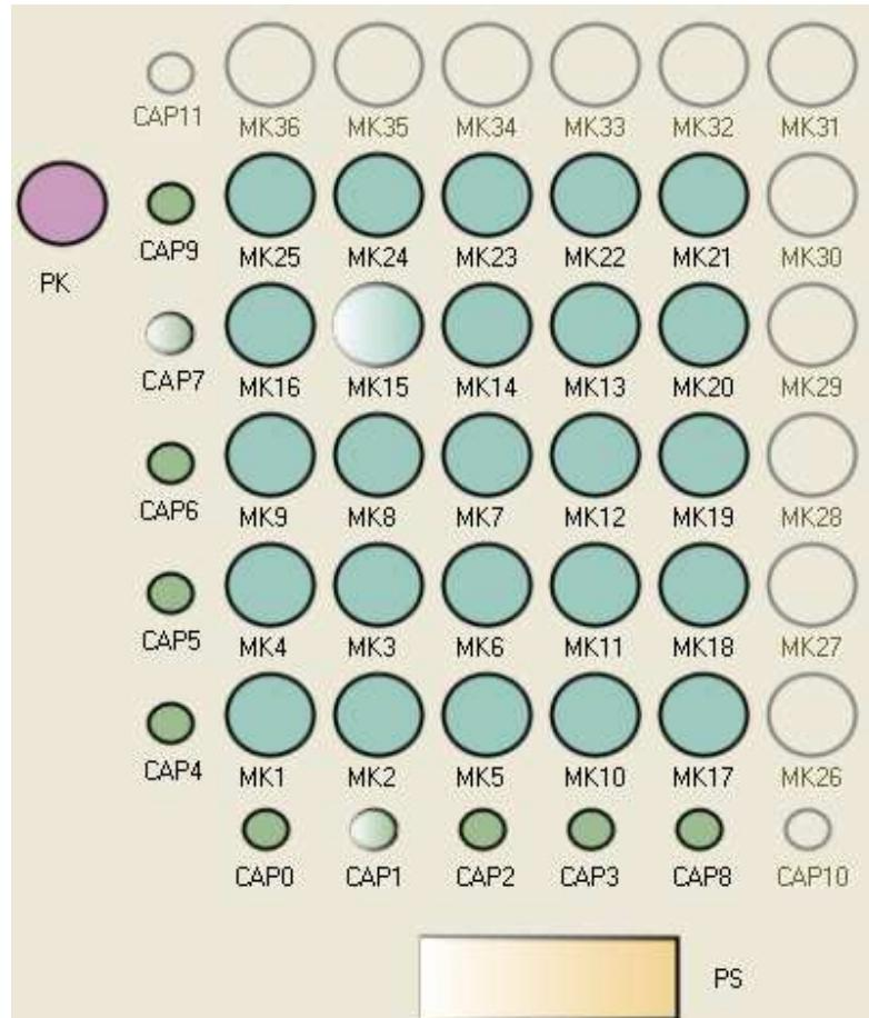
Figure 30: Example Proximity Detected and MK15 Touched.
