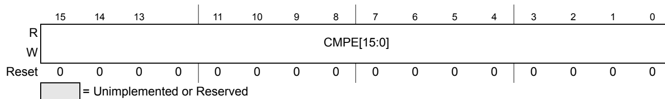
Figure 16-10. ATD Compare Enable Register (ATDCMPE)
