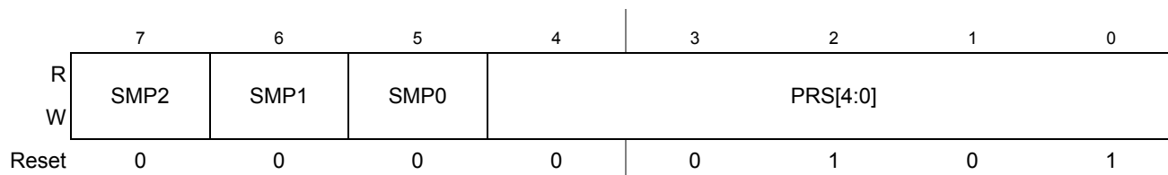
Figure 13-7. ATD Control Register 4 (ATDCTL4)
