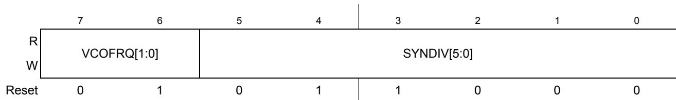
Figure 10-4. S12CPMU Synthesizer Register (CPMUSYNR)
