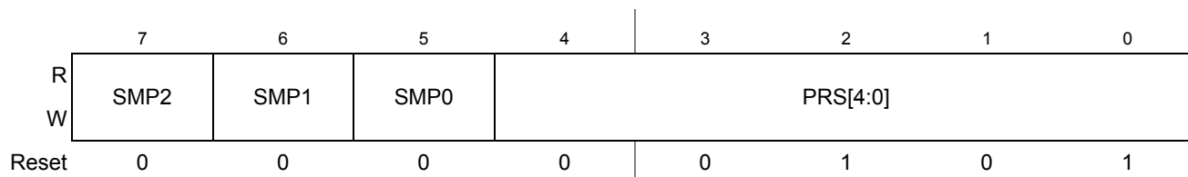
Figure 11-7. ATD Control Register 4 (ATDCTL4)
