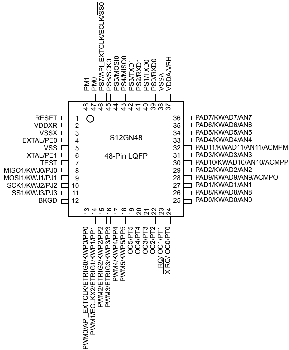
Figure 1-8. 48-Pin LQFP Pinout for S12GN48
