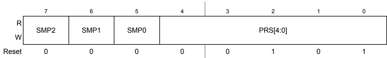
Figure 13-7. ATD Control Register 4 (ATDCTL4)
