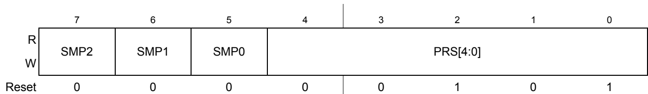
Figure 12-7. ATD Control Register 4 (ATDCTL4)
