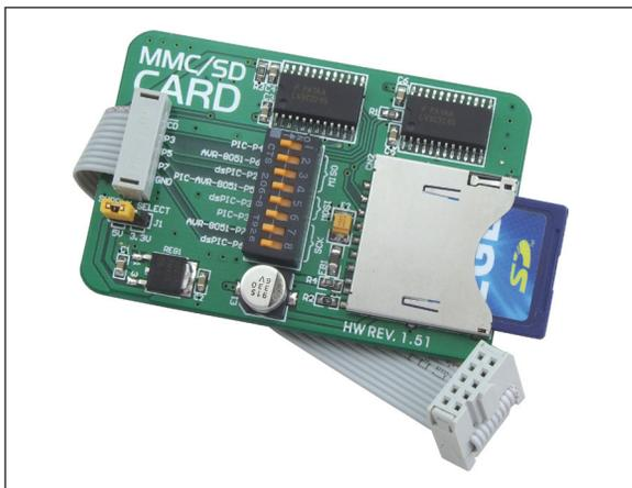
Figure 1: MMC/SD additional board
