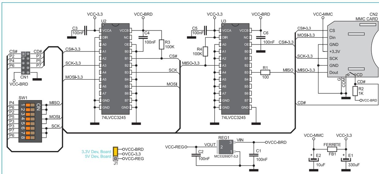
Figure 3: MMC/SD additional board connection schematic
