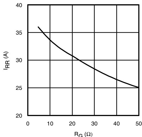
**Fig. 19 - Typ. Diode  $I_{RR}$  vs.  $R_G$**
