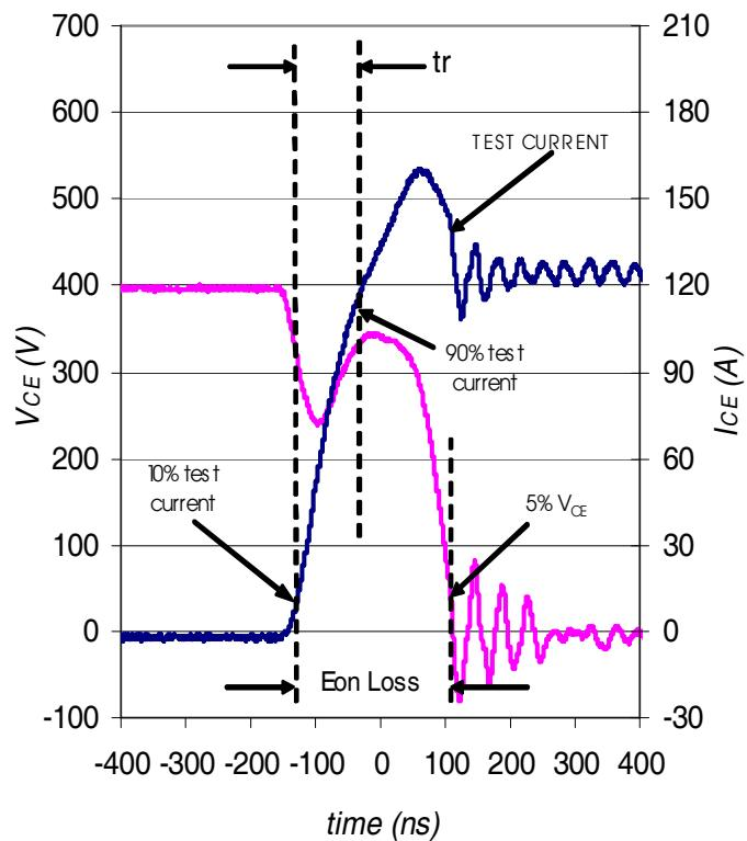
**Fig. WF2** - Typ. Turn-on Loss Waveform
