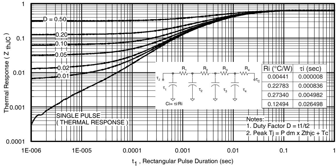
Fig. 27. Maximum Transient Thermal Impedance, Junction-to-Case (DIODE)
