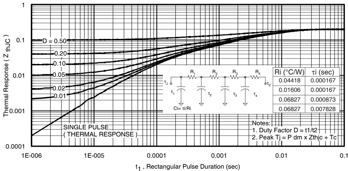
Fig 26. Maximum Transient Thermal Impedance, Junction-to-Case (IGBT)
