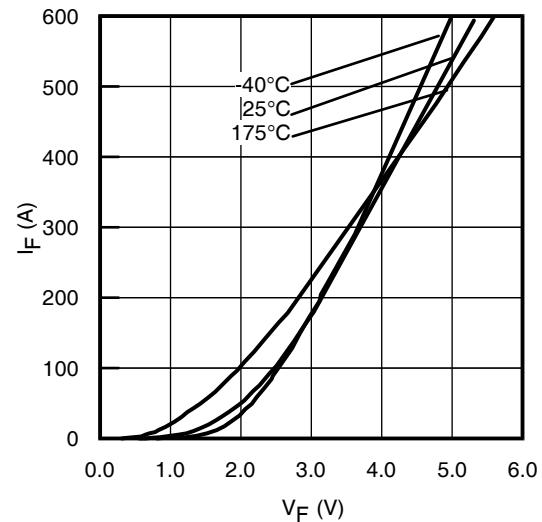
**Fig. 9** - Typ. Diode Forward Characteristics
