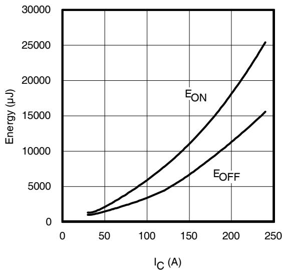
**Fig. 14** - Typ. Energy Loss vs.  $I_C$
