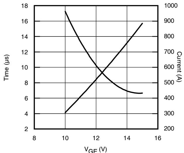
**Fig. 23 -  $V_{GE}$  vs. Short Circuit Time**
