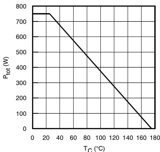
**Fig. 3 - Power Dissipation vs. Case Temperature**
