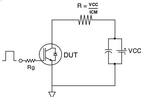
**Fig.C.T.5 - Resistive Load Circuit**
