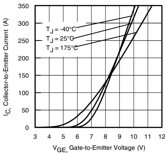
**Fig. 13** - Typ. Transfer Characteristics
