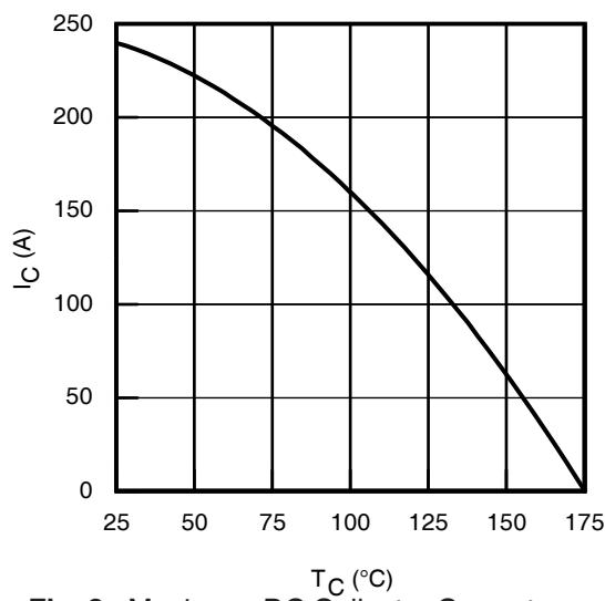
**Fig. 2 - Maximum DC Collector Current vs. Case Temperature**
