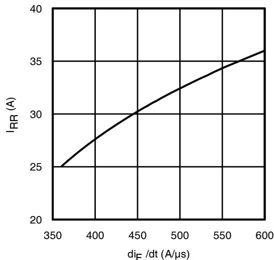
**Fig. 20 - Typ. Diode  $I_{RR}$  vs.  $dI_F/dt$**
