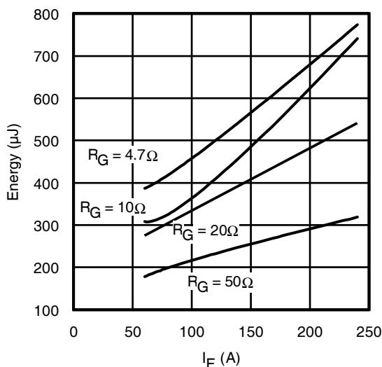
**Fig. 22 - Typ. Diode  $E_{RR}$  vs.  $I_F$**
