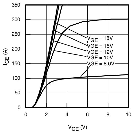
**Fig. 7** - Typ. IGBT Output Characteristics
