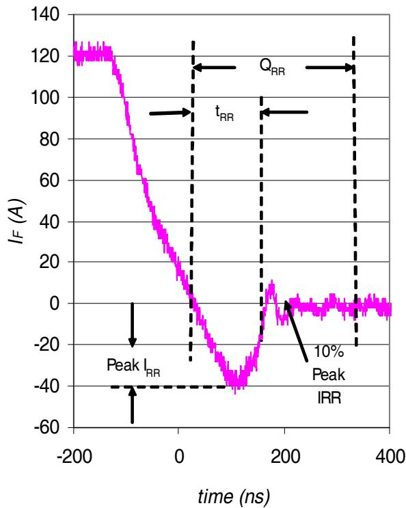
**Fig. WF3** - Typ. Diode Recovery Waveform
