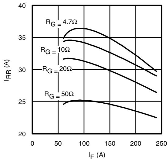
**Fig. 18 - Typ. Diode  $I_{RR}$  vs.  $I_F$**
