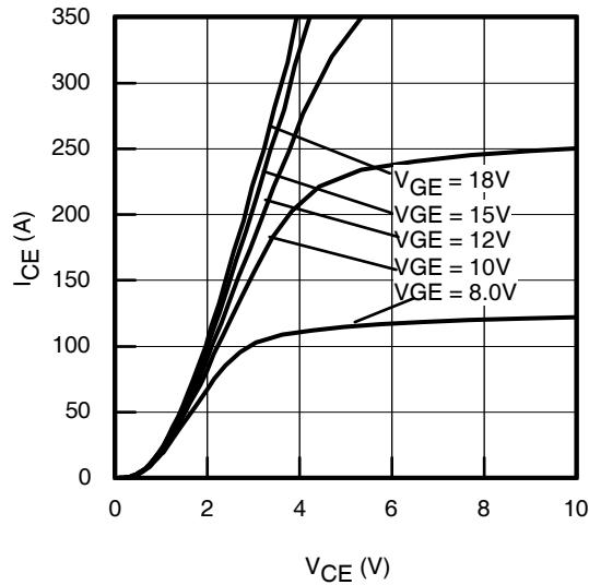
**Fig. 8** - Typ. IGBT Output Characteristics
