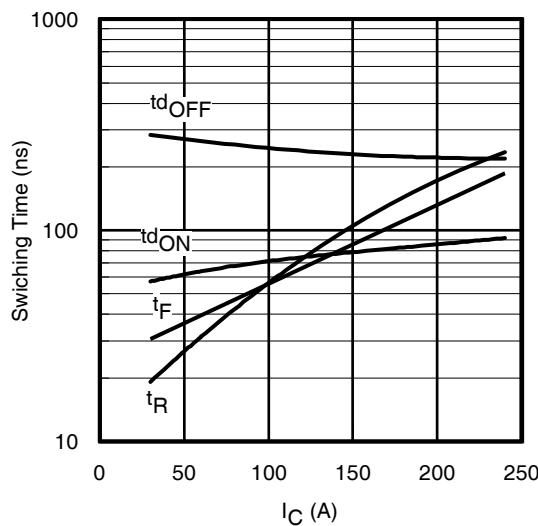
**Fig. 15** - Typ. Switching Time vs.  $I_C$
