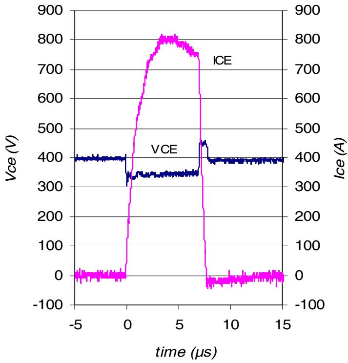
**Fig. WF4** - Typ. S.C. Waveform
