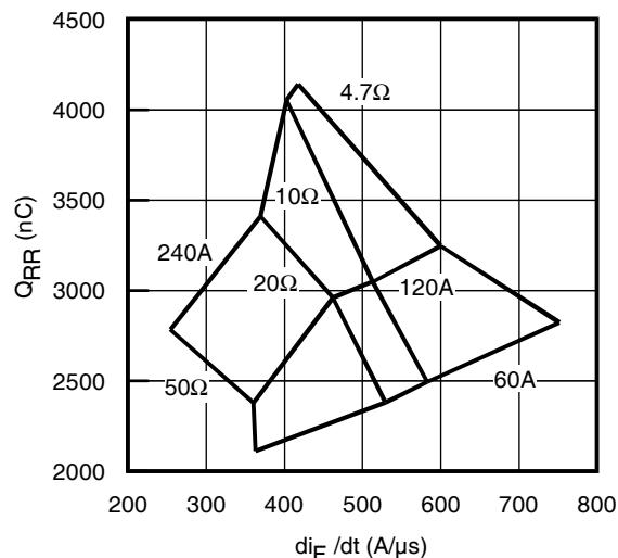
**Fig. 21 - Typ. Diode  $Q_{RR}$  vs.  $dI_F/dt$**
