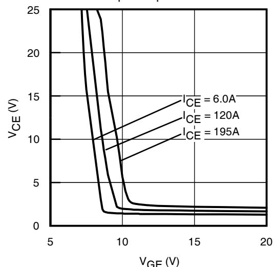
**Fig. 11** - Typical  $V_{CE}$  vs.  $V_{GE}$
