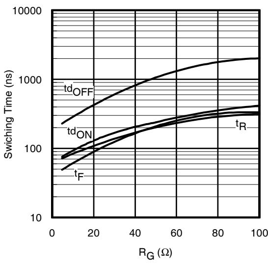
**Fig. 17** - Typ. Switching Time vs.  $R_G$
