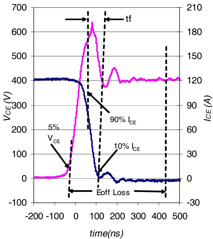
**Fig. WF1** - Typ. Turn-off Loss Waveform
