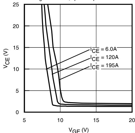
**Fig. 10** - Typical  $V_{CE}$  vs.  $V_{GE}$
