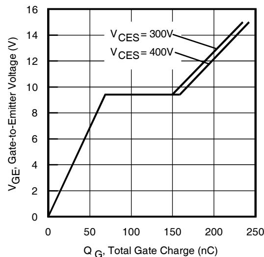
Fig. 25 - Typical Gate Charge vs.  $V_{GE}$
