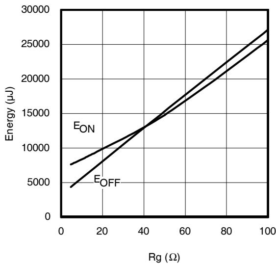
**Fig. 16** - Typ. Energy Loss vs.  $R_G$
