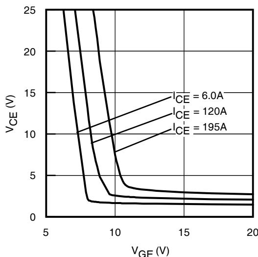
**Fig. 12** - Typical  $V_{CE}$  vs.  $V_{GE}$
