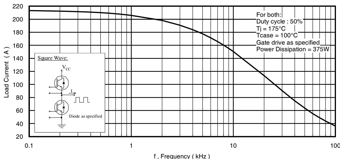
**Fig. 1 - Typical Load Current vs. Frequency**
