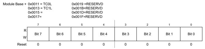
Figure 11-19. Timer Input Capture/Output Compare Register x Low (TCxL)
