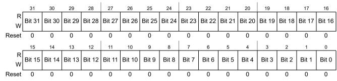
Figure 6-14. Debug Comparator A Data Mask Register (DBGADM)
