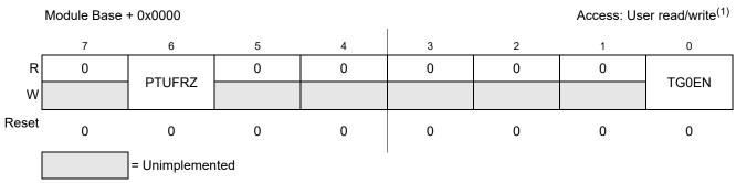
Figure 13-3. PTU Module Enable Register (PTUE)
