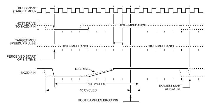
Figure 5-7. BDC Target-to-Host Serial Bit Timing (Logic 1)
