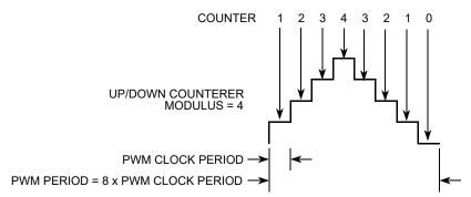
Figure 12-44. Center-Aligned PWM Period
