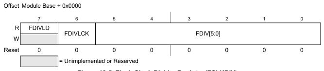
Figure 18-5. Flash Clock Divider Register (FCLKDIV)
