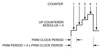
Figure 12-45. Edge-Aligned PWM Period
