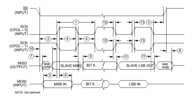
Figure H-5. SPI Slave Timing (CPHA=0)
