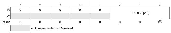
Figure 4-8. Interrupt Request Configuration Data Register 3 (INT\_CFDATA3) 1. Please refer to the notes following the PRIOLVL[2:0] description below.
