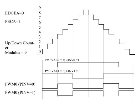
Figure 12-65. Double-Switching PWM Output VAL0<VAL1 (Center-Aligned)
