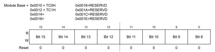
Figure 11-18. Timer Input Capture/Output Compare Register x High (TCxH)
