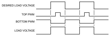
Figure 12-61. Correction with Negative Current
