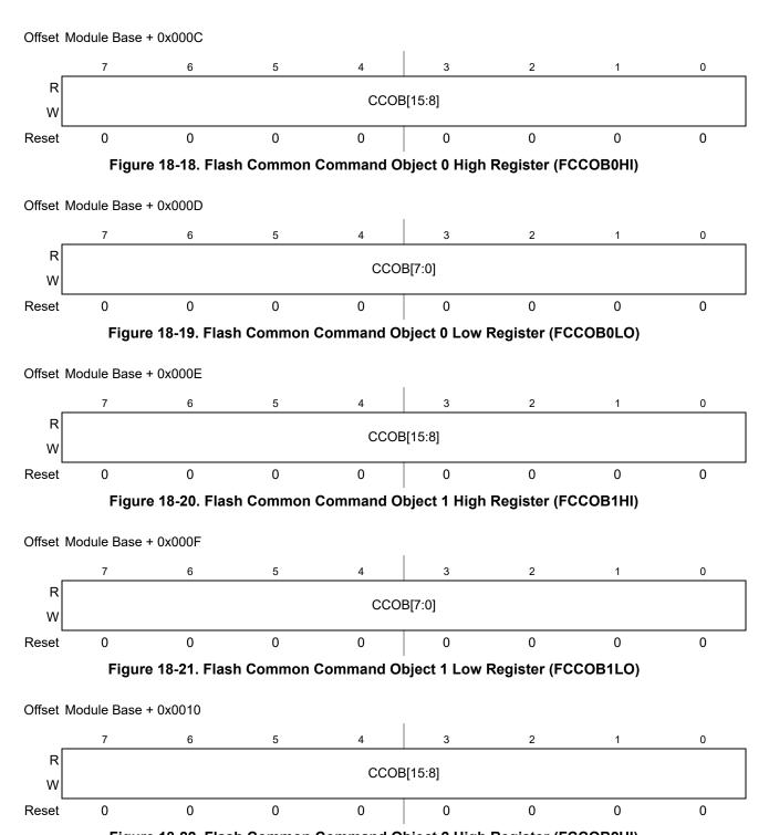
Figure 18-22. Flash Common Command Object 2 High Register (FCCOB2HI)
