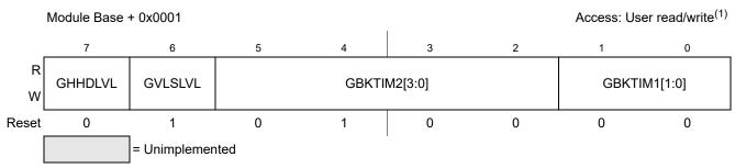
Figure 17-4. GDU1PHV1 Control Register (GDUCTR)
