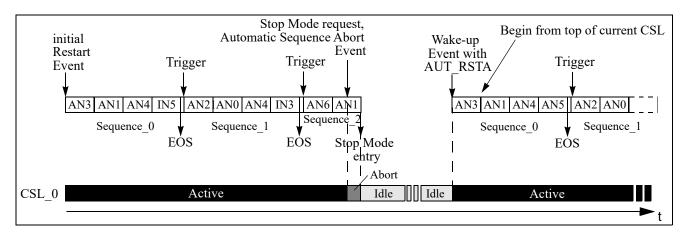
Figure 9-43. Conversion Flow Control Diagram — Triggered Conversion (with Stop Mode)
