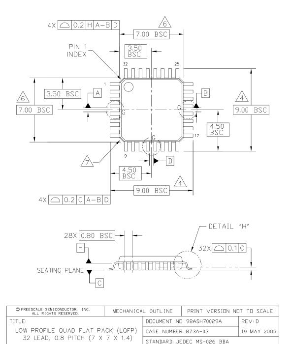
Figure I-3. 32LQFP Mechanical Information (1 of 3)
