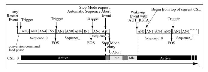
Figure 9-44. Conversion Flow Control Diagram — Fully Timing Controlled Conversion (with Stop Mode)
