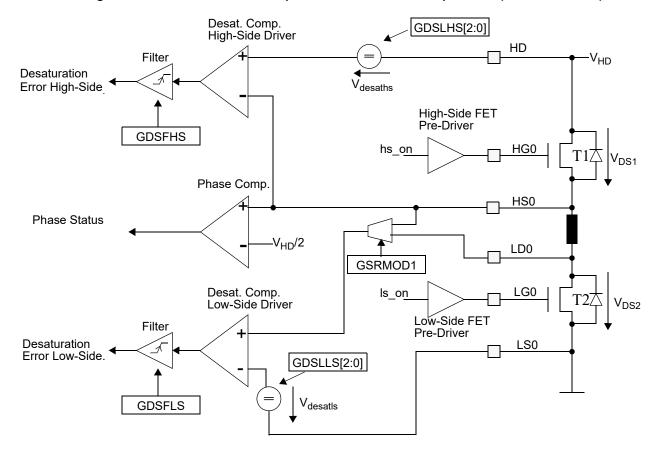
Figure 17-23. Desaturation Comparators and Phase Comparators (LD0 connected)
