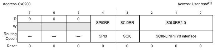
Figure 2-1. Module Routing Register 0 (MODRR0)
