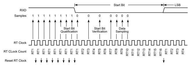
Figure 14-21. Receiver Data Sampling
