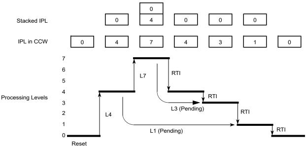
Figure 4-14. Interrupt Processing Example
