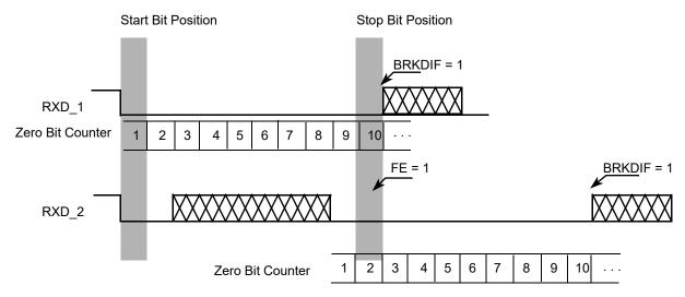
Figure 14-17. Break Detection if BRKDFE = 1 (M = 0)
