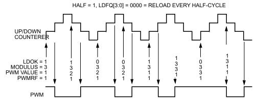
Figure 12-78. Half-Cycle Center-Aligned PWM Value Loading
