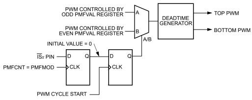
Figure 12-59. Internal Correction Logic when ISENS = 11
