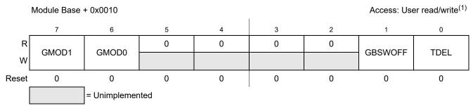
Figure 17-18. GDU Control Register 1 (GDUCTR1)
