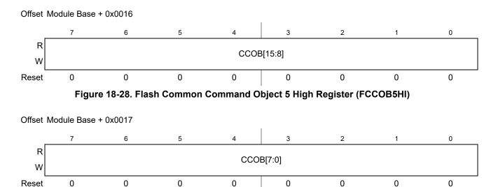
Figure 18-29. Flash Common Command Object 5 Low Register (FCCOB5LO)
