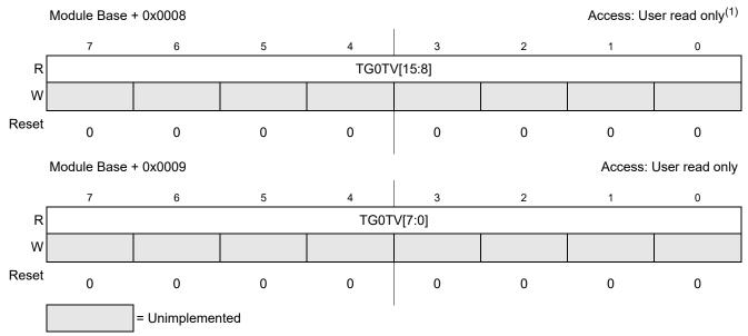
Figure 13-11. Trigger Generator 0 Trigger Value Register (TG0TVH, TG0TVL)
