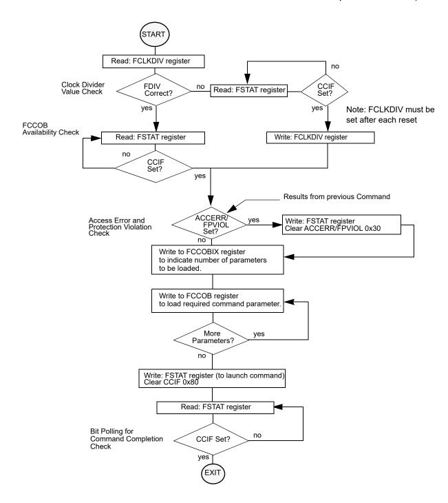
Figure 18-30. Generic Flash Command Write Sequence Flowchart
