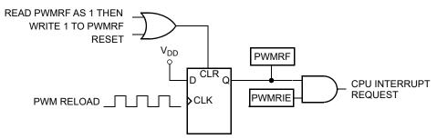
Figure 12-75. PWMRF Reload Interrupt Request
