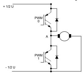
Figure 1-9. DC Brushed Motor External Configuration
