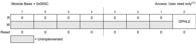
Figure 17-15. GDU Phase Log Register (GDUPHL)
