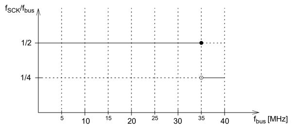
Figure H-4. Derating of maximum  $f_{\mbox{\footnotesize SCK}}$  to  $f_{\mbox{\footnotesize bus}}$  ratio in Master Mode
