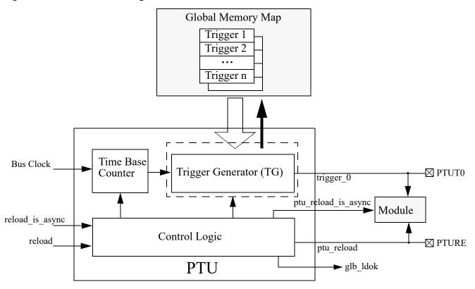
Figure 13-1. PTU Block Block Diagram
