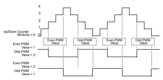
Figure 12-62. Asymmetric Waveform - Phase Shift PWM Output
