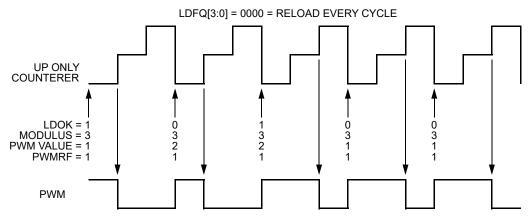
Figure 12-80. Edge-Aligned PWM Value Loading
