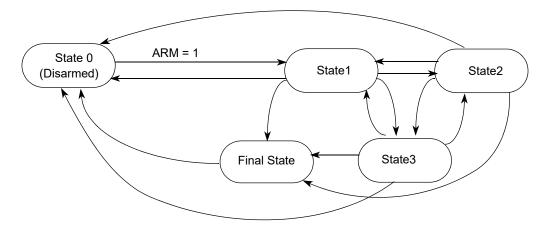
Figure 6-19. State Sequencer Diagram
