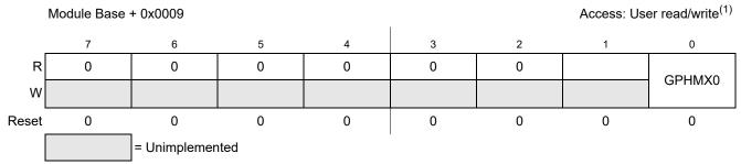
Figure 17-12. GDU Phase Mux Register (GDUPHMUX)
