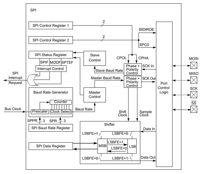
Figure 15-1. SPI Block Diagram
