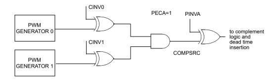
Figure 12-63. Logic AND Function with Signal Inversions
