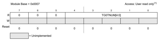
Figure 13-10. Trigger Generator 0 Trigger Number Register (TG0TNUM)
