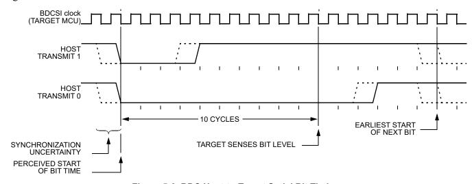
Figure 5-6. BDC Host-to-Target Serial Bit Timing
