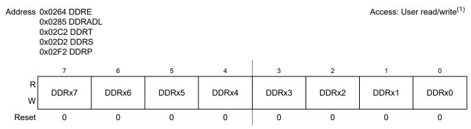
Figure 2-15. Data Direction Register
