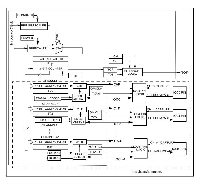
Figure 11-22. Detailed Timer Block Diagram
