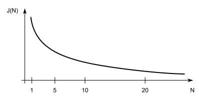
Figure B-2. Maximum Bus Clock Jitter Approximation (N = number of bus cycles)
