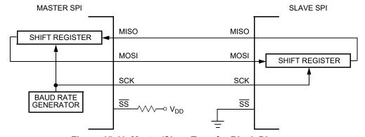
Figure 15-11. Master/Slave Transfer Block Diagram
