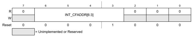
Figure 4-4. Interrupt Configuration Address Register (INT\_CFADDR)
