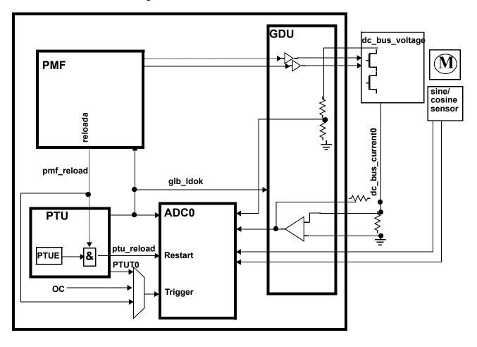
Figure 1-5. Motor Control Module interfaces
