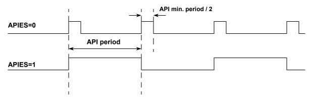
Figure 8-23. Waveform selected on API\_EXTCLK pin (APIEA=1, APIFE=1)
