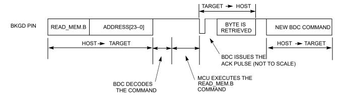
Figure 5-10. Handshake Protocol at Command Level
