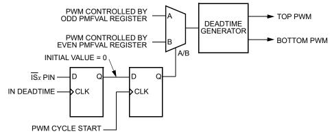
Figure 12-58. Internal Correction Logic when ISENS = 10
