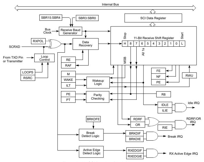
Figure 14-20. SCI Receiver Block Diagram
