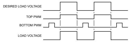
Figure 12-60. Correction with Positive Current
