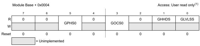
Figure 17-7. GDU1PHV1 Status Register (GDUSTAT)
