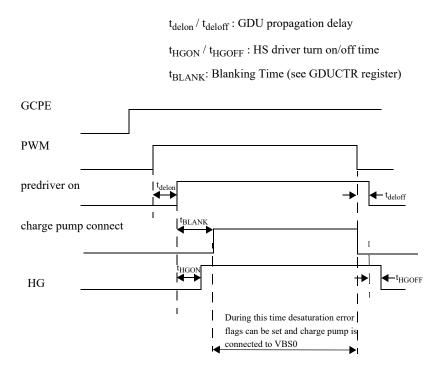
Figure 17-20. Timing Diagram Charge Pump Connect
