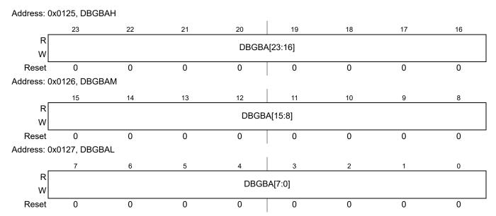
Figure 6-16. Debug Comparator B Address Register
