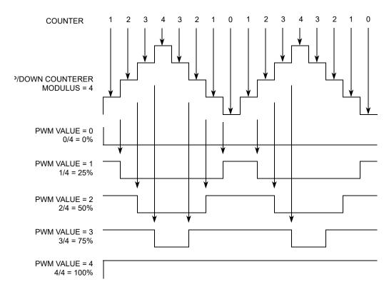
Figure 12-46. Center-Aligned PWM Pulse Width
