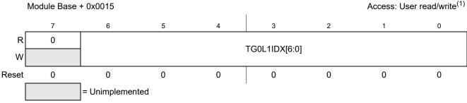
Figure 13-15. Trigger Generator 0 List 1 Index (TG0L1IDX)
