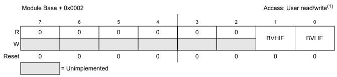
Figure 10-6. BATS Interrupt Enable Register (BATIE)
