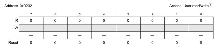
Figure 2-4. Module Routing Register 2 (MODRR2)
