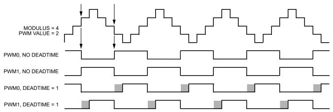
Figure 12-51. Deadtime Insertion, Center Alignment
