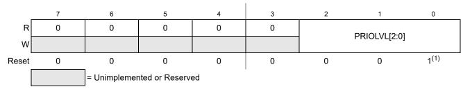
Figure 4-9. Interrupt Request Configuration Data Register 4 (INT\_CFDATA4)
