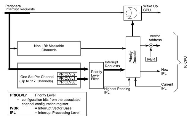
Figure 4-1. S12ZINT Block Diagram
