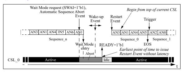
Figure 9-1. Conversion Flow Control Diagram - Wait Mode (SWAI=1'b1, AUT RSTA=1'b0)
