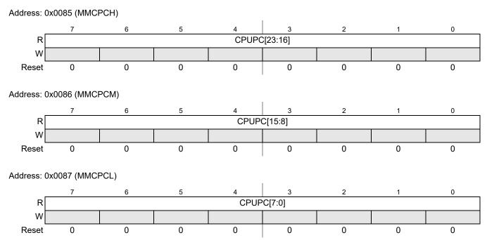
Figure 3-7. Captured S12ZCPU Program Counter (MMCPCH, MMCPCM, MMCPCL)
