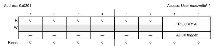
Figure 2-3. Module Routing Register 1 (MODRR1)
