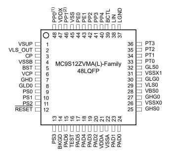
Figure 1-3. MC9S12ZVMA-Family 48-pin LQFP pin out
