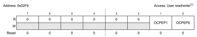
Figure 2-26. Over-Current Protection Enable Register (OCPEP)
