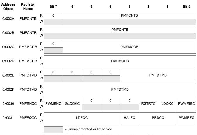
Figure 12-2. Quick Reference to PMF Registers (Sheet 4 of 5)
