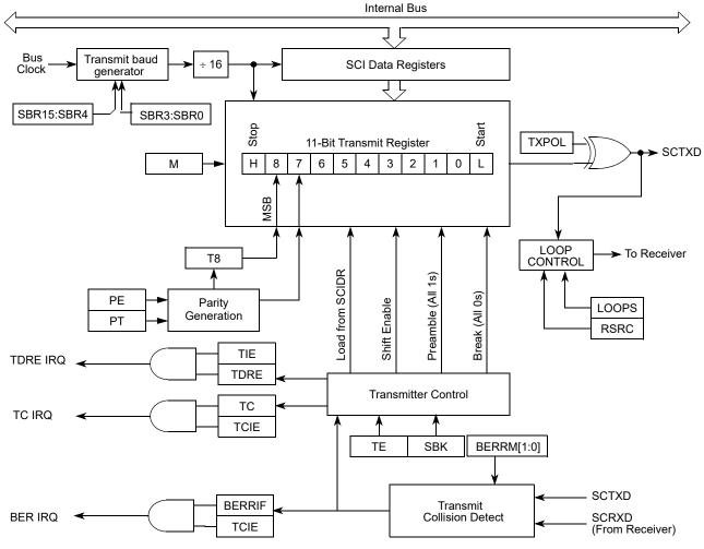
Figure 14-16. Transmitter Block Diagram
