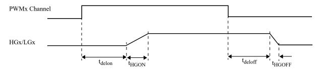
Figure 17-30 shows examples of intrinsic dead times. For example assuming minimum values for  $t_{\rm HGON}$  and  $t_{\rm delon}$  for the high side gate HG0 and minimum values for  $t_{\rm HGOFF}$  and  $t_{\rm deloff}$  for low-side gate LG0 no additional dead time setting in the PMF module is required and the PWM channels can change at the same time without cross conduction of the power MOSFETs.
