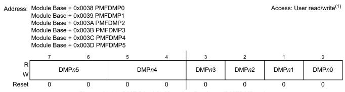
Figure 12-39. PMF Disable Mapping Register (PMFDMP0-5)
