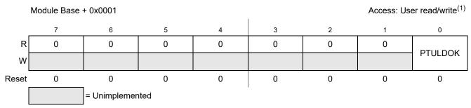
Figure 13-4. PTU Module Control Register (PTUC)
