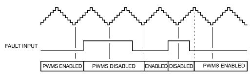
Figure 12-83. Automatic Fault Recovery
