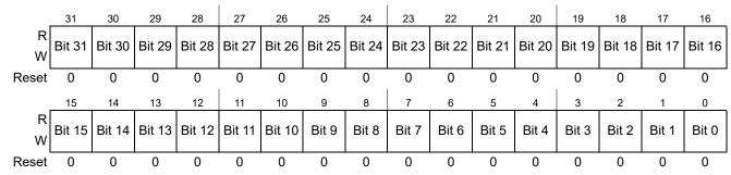
Figure 6-13. Debug Comparator A Data Register (DBGAD)
