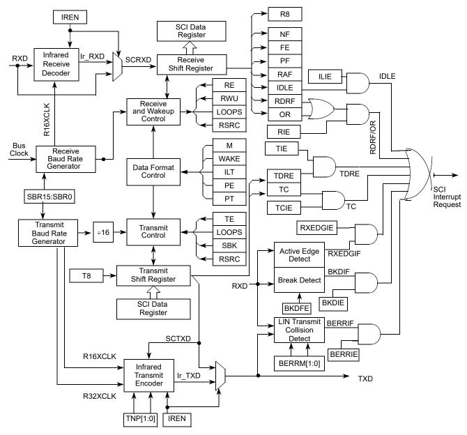
Figure 14-14. Detailed SCI Block Diagram
