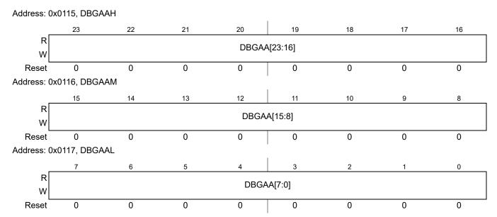
Figure 6-12. Debug Comparator A Address Register
