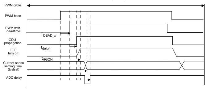
Figure 1-11. Control Loop Delay Overview
