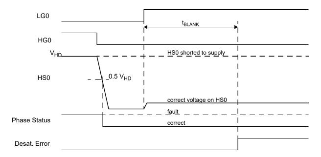
Figure 17-25. Short to Ground Detection
