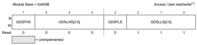
Figure 17-14. GDU Desaturation Level Register (GDUDSLVL)
