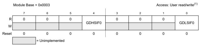
Figure 17-6. GDU1PHV1 Desaturation Error Flag Register (GDUDSE)
