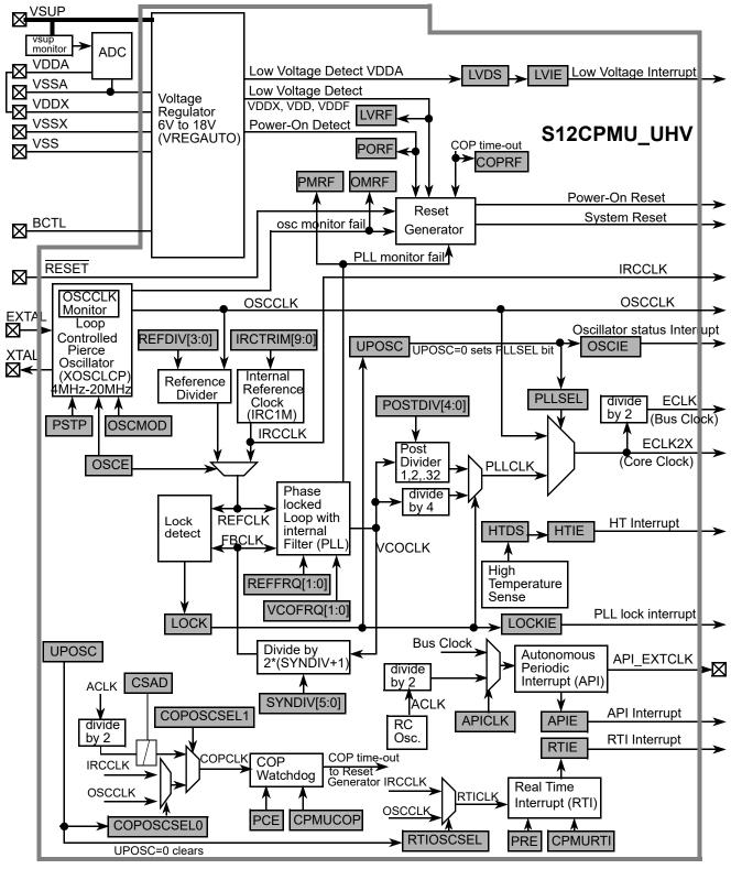
Figure 8-1. Block diagram of S12CPMU\_UHV\_V11
