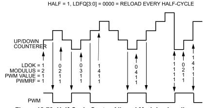
Figure 12-79. Half-Cycle Center-Aligned Modulus Loading
