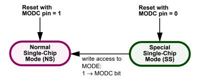
Figure 3-4. Mode Transition Diagram
