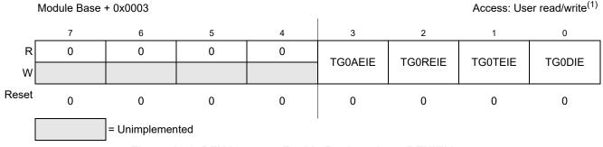
Figure 13-6. PTU Interrupt Enable Register Low (PTUIEL)
