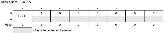
Figure 8-33. S12CPMU\_UHV\_V11 Oscillator Register (CPMUOSC)
