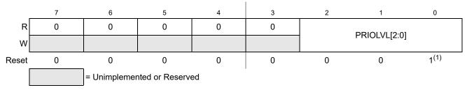
Figure 4-12. Interrupt Request Configuration Data Register 7 (INT\_CFDATA7)
