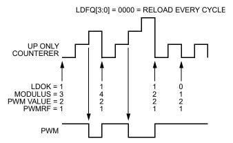
Figure 12-81. Edge-Aligned Modulus Loading
