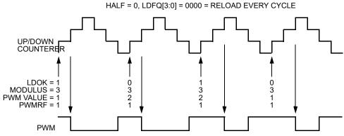
Figure 12-76. Full-Cycle Center-Aligned PWM Value Loading
