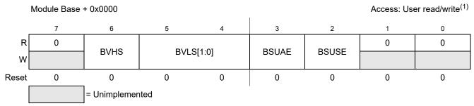
Figure 10-3. BATS Module Enable Register (BATE)
