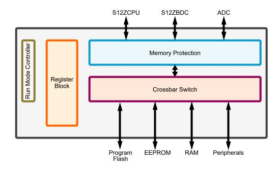
Figure 3-1. S12ZMMC Block Diagram
