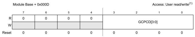
Figure 17-16. GDU Clock Control Register 2 (GDUCLK2)
