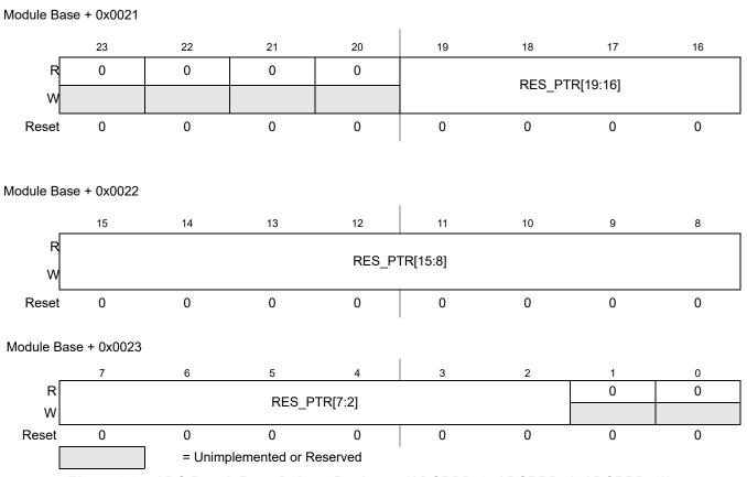
Figure 9-25. ADC Result Base Pointer Registers (ADCRBP\_0, ADCRBP\_1, ADCRBP\_2))
