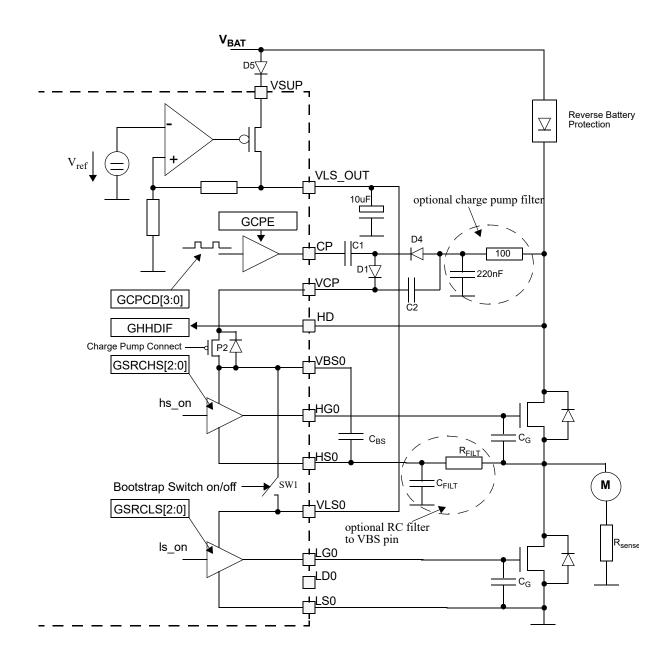
Figure 17-19. FET Pre-Driver Circuit and Voltage Regulator
