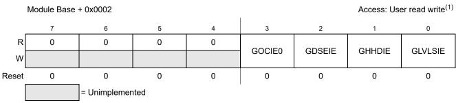
Figure 17-5. GDU1PHV1 Interrupt Enable Register (GDUIE)
