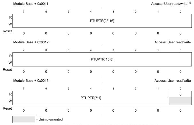
Figure 13-13. PTU List Add Register (PTUPTRH, PTUPTRM, PTUPTRL)
