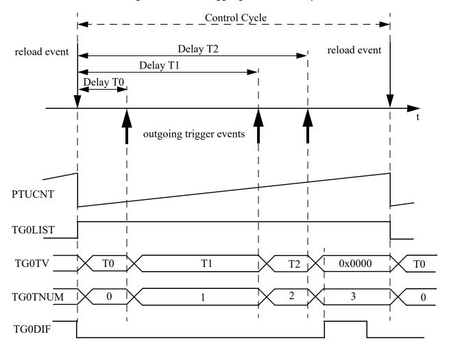
Figure 13-17. TG0 trigger generation example
