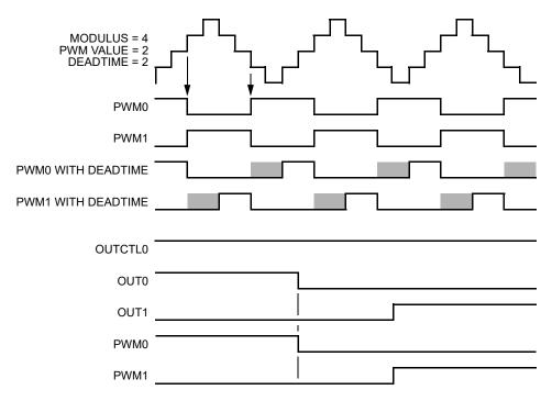
Figure 12-69. Clearing OUT0 with OUTCTL Set in Complementary Mode
