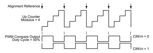
Figure 12-43. Edge-Aligned PWM Output
