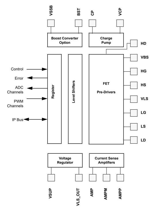
Figure 17-1. GDU Block Diagram
