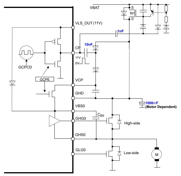
Figure 1-13. High-side Supply and Charge Pump Concept
