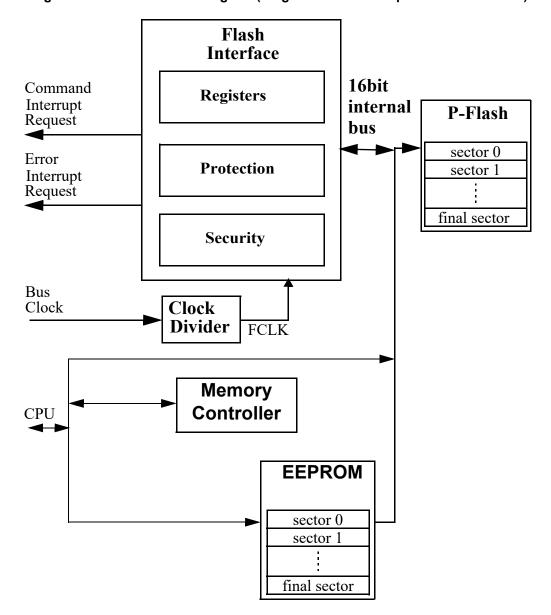
Figure 18-1. FTMRZ Block Diagram (Single P-Flash Block plus EEPROM block)
