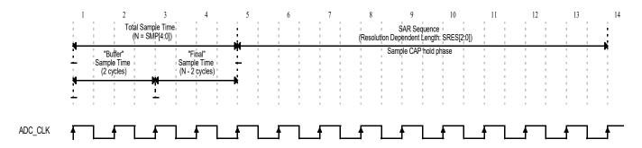
Figure 9-28. Sampling and Conversion Timing Example (8-bit Resolution, 4 Cycle Sampling)
