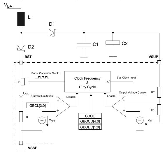
Figure 17-27. Boost Converter Option with external Components<sup>1</sup>
