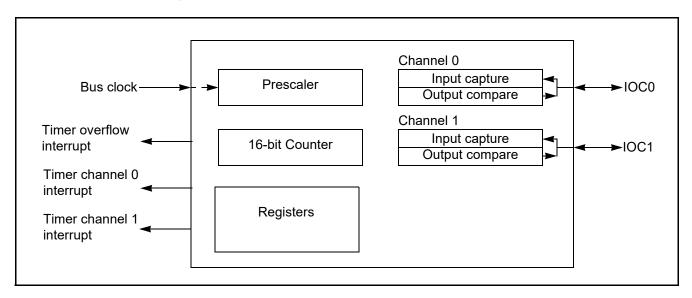
Figure 11-1. TIM16B2CV3 Block Diagram
