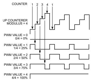
Figure 12-47. Edge-Aligned PWM Pulse Width
