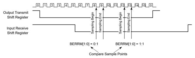
Figure 14-19. Timing Diagram Bit Error Detection
