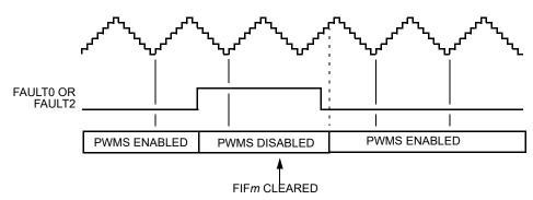
Figure 12-84. Manual Fault Recovery (Faults 0 and 2) — QSMP = 00
