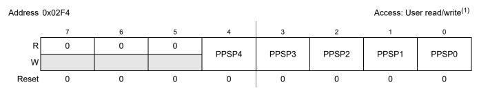
Figure 2-25. Port P Polarity Select Register (PPSP)
