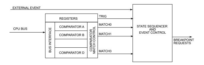
Figure 6-1. Debug Module Block Diagram
