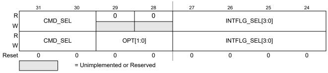
Figure 9-18. ADC Command Register 0 (ADCCMD\_0)
