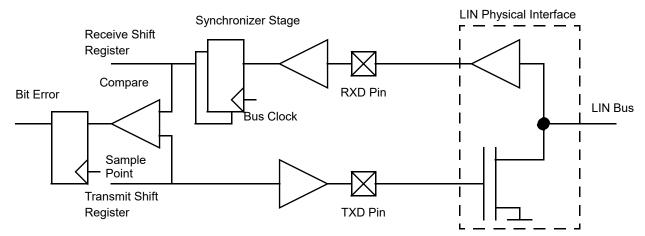
Figure 14-18. Collision Detect Principle
