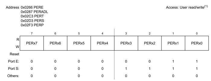
Figure 2-16. Pull Device Enable Register
