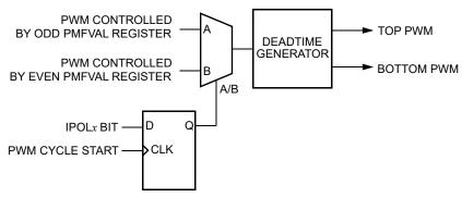
Figure 12-55. Internal Correction Logic when ISENS = 01
