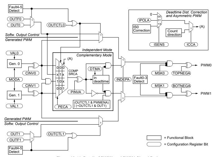
Figure 12-41. Detail of PWM0 and PWM1 Signal Paths
