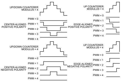
Figure 12-67. PWM Polarity
