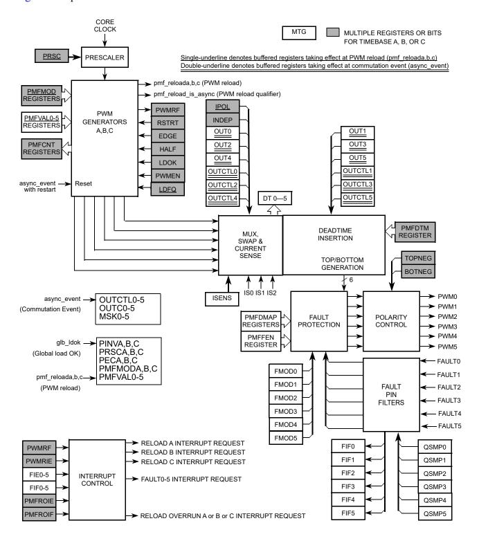
Figure 12-1. PMF Block Diagram
