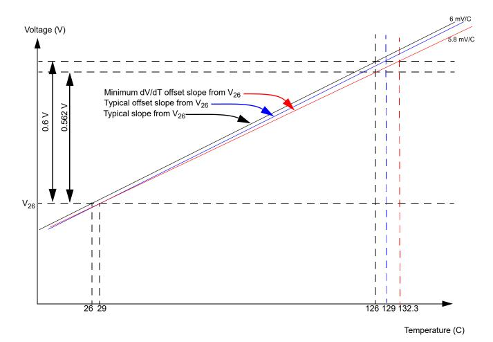
Figure 1-8. Effect of slope plus V<sub>26</sub> reference inaccuracy
