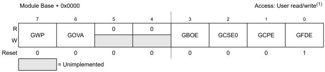
Figure 17-3. GDU1PHV1 Module Enable Register (GDUE)
