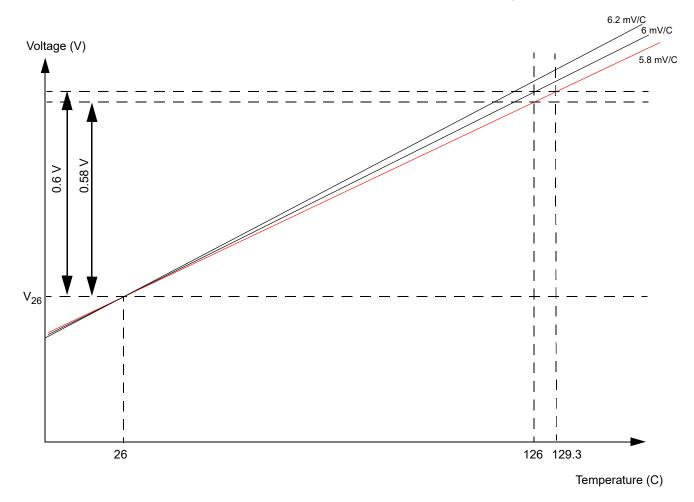
Figure 1-7. DVBE effect of slope inaccuracy
