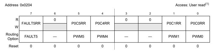
Figure 2-6. Module Routing Register 4 (MODRR4)
