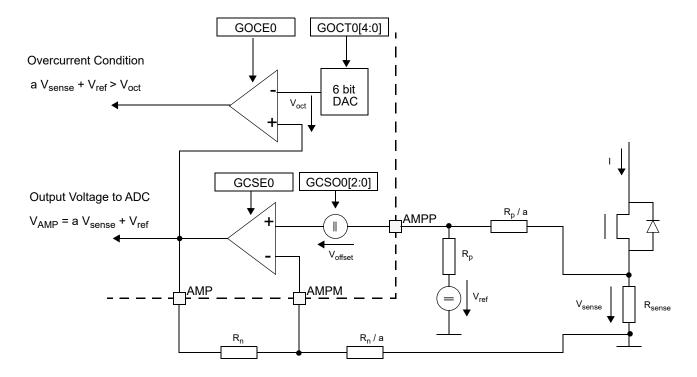
Figure 17-26. Current Sense Amplifier Connected as Differential Amplifier
