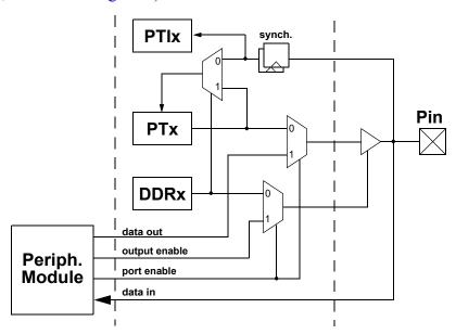
Figure 2-29. Illustration of I/O pin functionality
