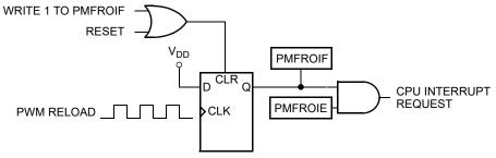
Figure 12-82. PMFROIF Reload Overrun Interrupt Request
