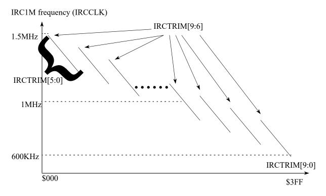
Figure 8-31. IRC1M Frequency Trimming Diagram
