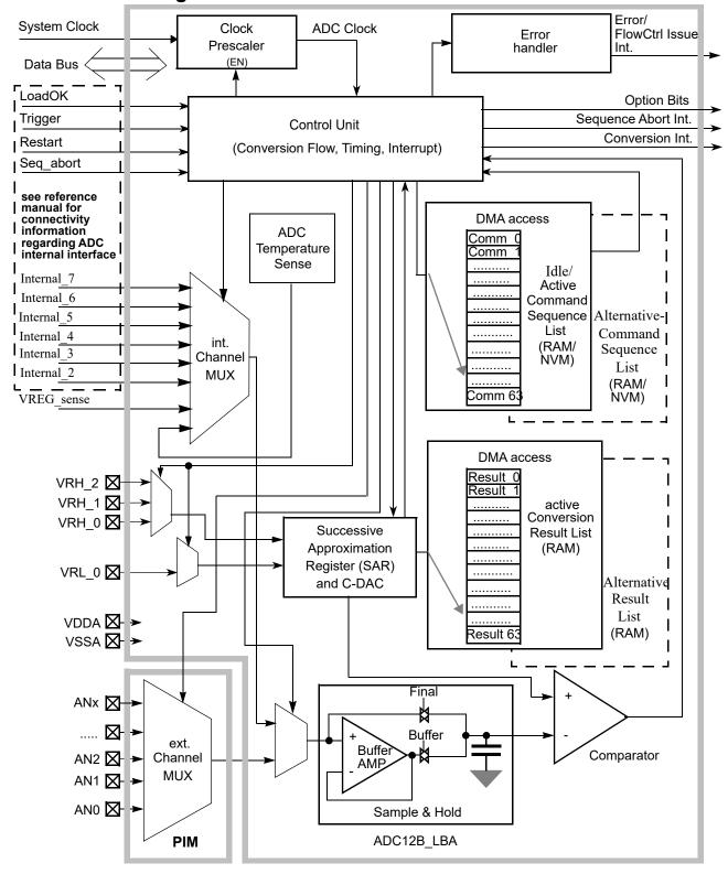
Figure 9-2. ADC12B\_LBA Block Diagram
