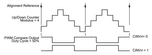
Figure 12-42. Center-Aligned PWM Output
