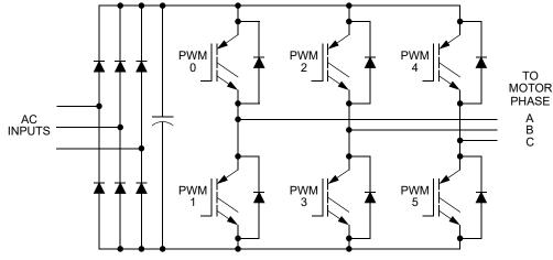
Figure 12-49. Typical 3-Phase AC Motor Drive
