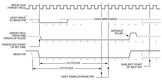
Figure 5-8. BDC Target-to-Host Serial Bit Timing (Logic 0)
