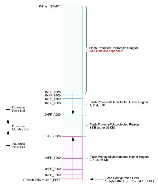
Figure 18-2. P-Flash Memory Map With Protection Alignment
