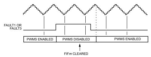
Figure 12-86. Manual Fault Recovery (Faults 1 and 3-5)
