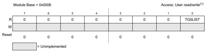
Figure 13-9. Trigger Generator 0 List Register (TG0LIST)
