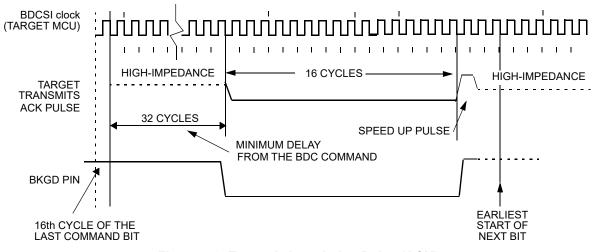
Figure 5-9. Target Acknowledge Pulse (ACK)
