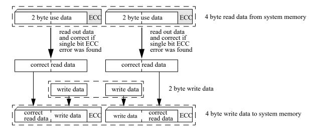
Figure 7-9. 2 byte non-aligned write access
