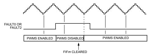
Figure 12-85. Manual Fault Recovery (Faults 0 and 2) — QSMP = 01, 10, or 11
