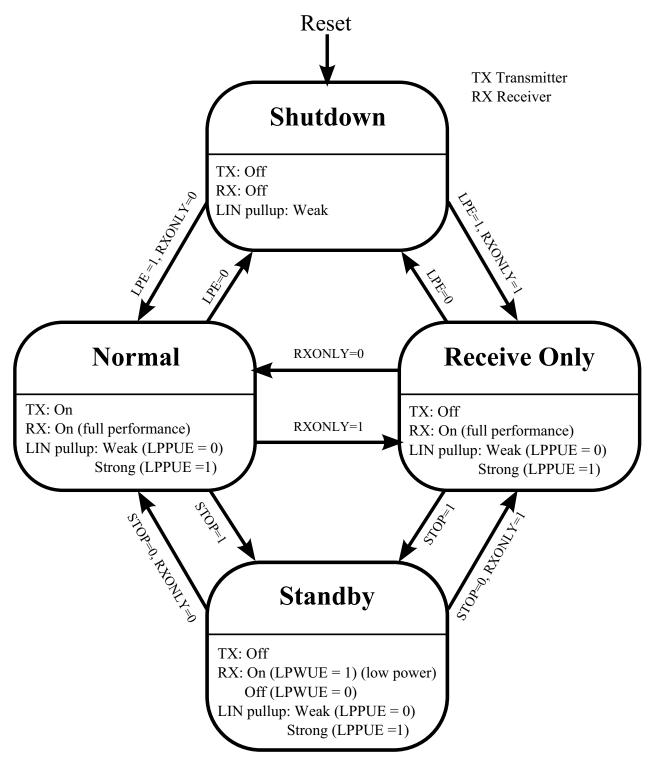
Figure 16-11. LIN/HV Physical Layer Mode Transitions
