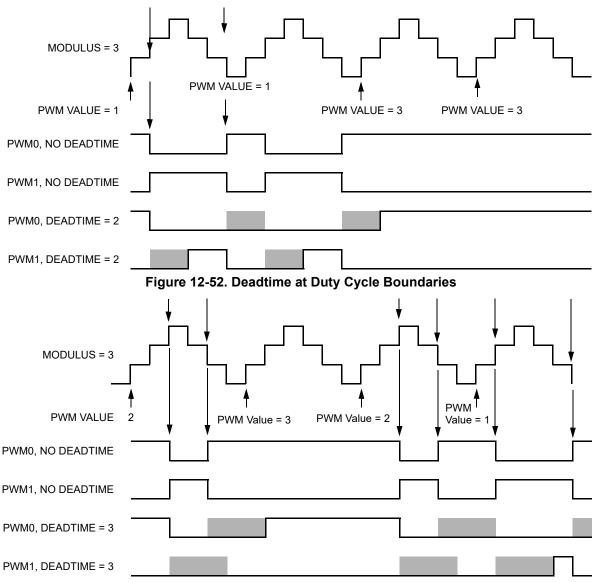
Figure 12-53. Deadtime and Small Pulse Widths
