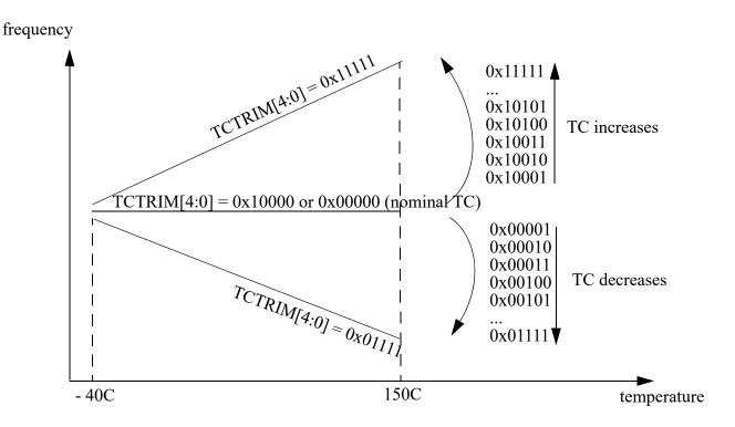
Figure 8-32. Influence of TCTRIM[4:0] on the Temperature Coefficient
