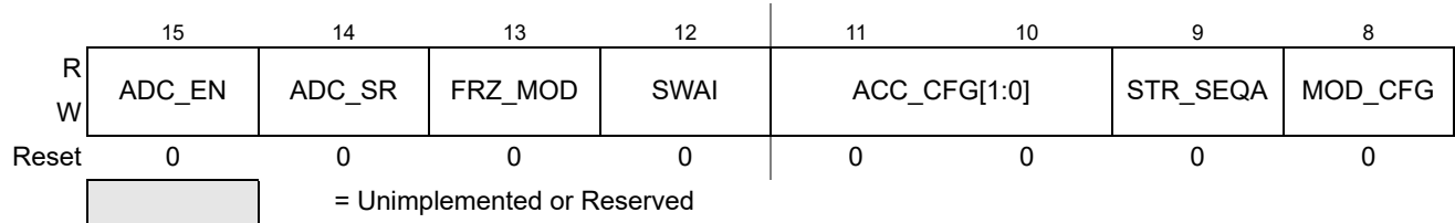
Figure 9-4. ADC Control Register 0 (ADCCTL_0)
