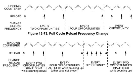
Figure 12-74. Half Cycle Reload Frequency Change
