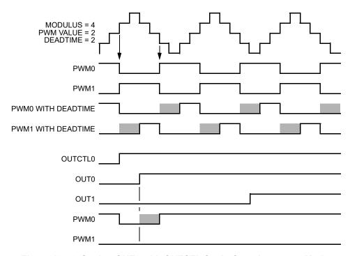
Figure 12-68. Setting OUT0 with OUTCTL Set in Complementary Mode
