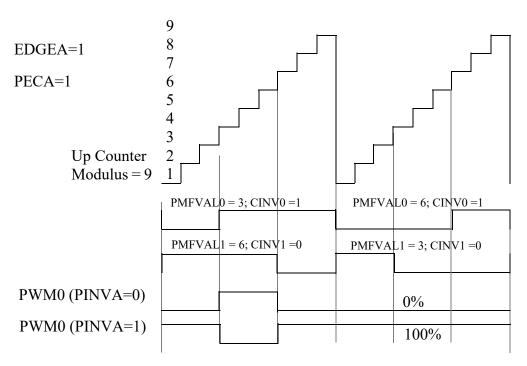
Figure 12-64. Variable Edge Placement Waveform - Phase Shift PWM Output (Edge-Aligned)
