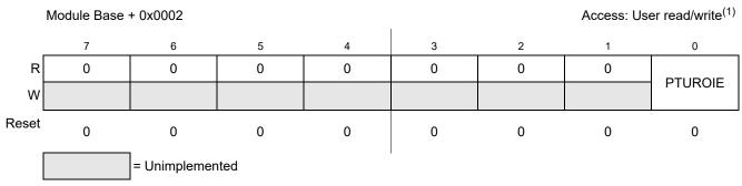
Figure 13-5. PTU Interrupt Enable Register High (PTUIEH)
