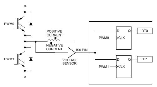
Figure 12-56. Current Status Sense Scheme for Deadtime Correction
