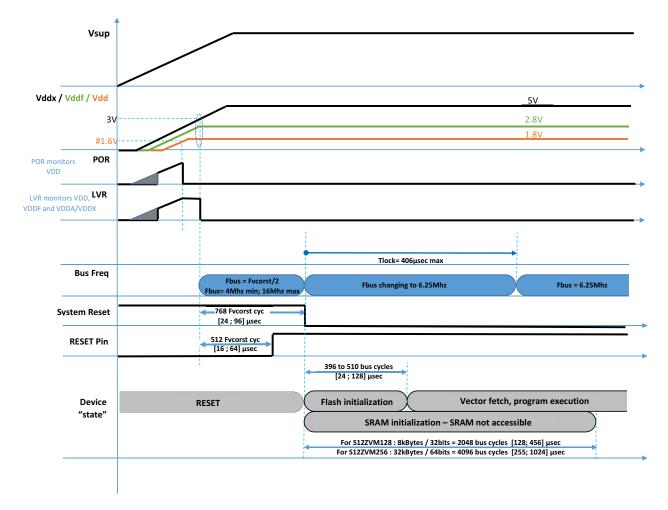
Figure 1-6. Device Power On Reset Sequence
