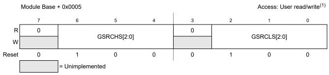
Figure 17-8. GDU Slew Rate Control Register (GDUSRC)
