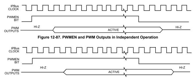
Figure 12-88. PWMEN and PWM Outputs in Complementary Operation
