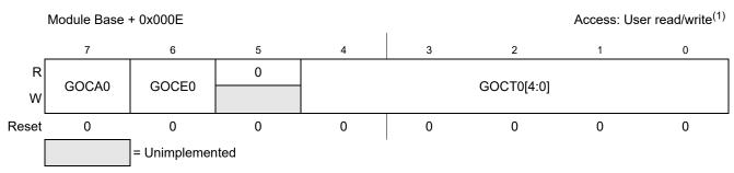
Figure 17-17. GDU Overcurrent Register 0 (GDUOC0)
