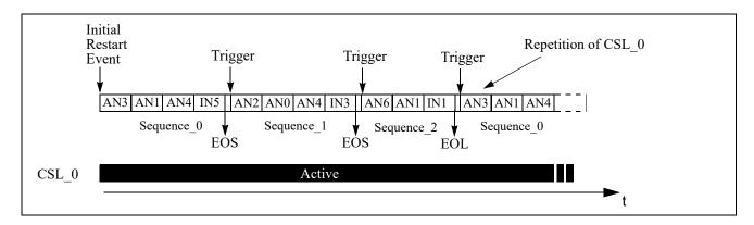
Figure 9-42. Conversion Flow Control Diagram — Triggered Conversion (CSL Repetition)
