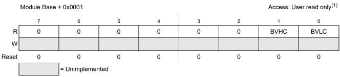
Figure 10-4. BATS Module Status Register (BATSR)
