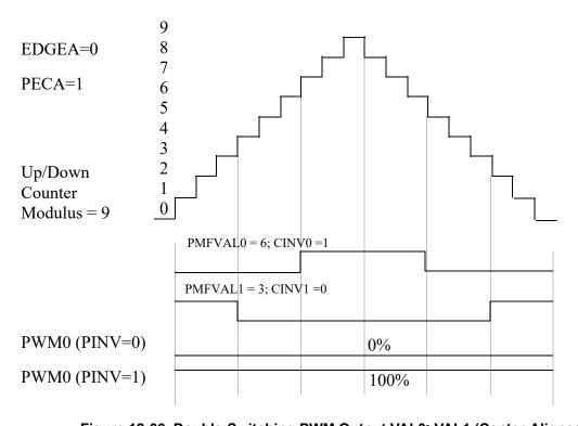
Figure 12-66. Double-Switching PWM Output VAL0>VAL1 (Center-Aligned)
