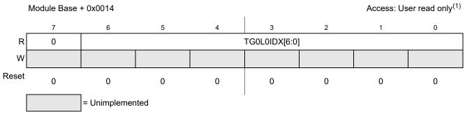
Figure 13-14. Trigger Generator 0 List 0 Index (TG0L0IDX)
