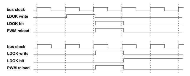
Figure 12-71. Setting cleared LDOK bit at PWM reload event
