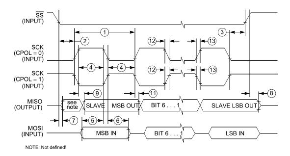
Figure H-6. SPI Slave Timing (CPHA=1)
