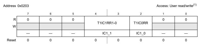
Figure 2-5. Module Routing Register 3 (MODRR3)
