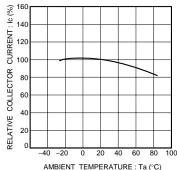
Fig.6 Relative output vs. ambient temperature
