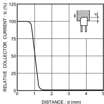
Fig.4 Relative output current vs. distance (II)
