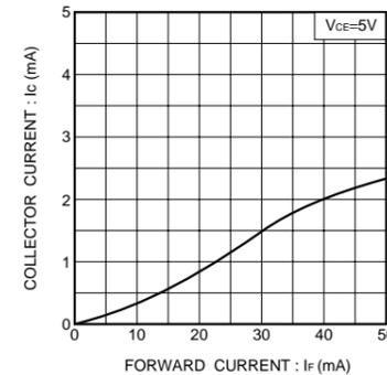
Fig.7 Collector current vs. forward current
