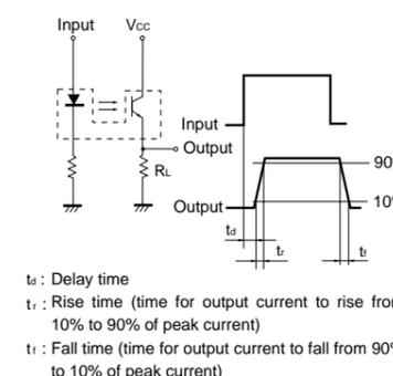
Fig.11 Response time measurement circuit
