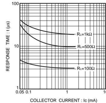
Fig.8 Response time vs. collector current
