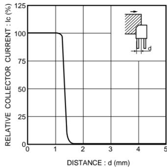
Fig.1 Relative output current vs. distance (I)
